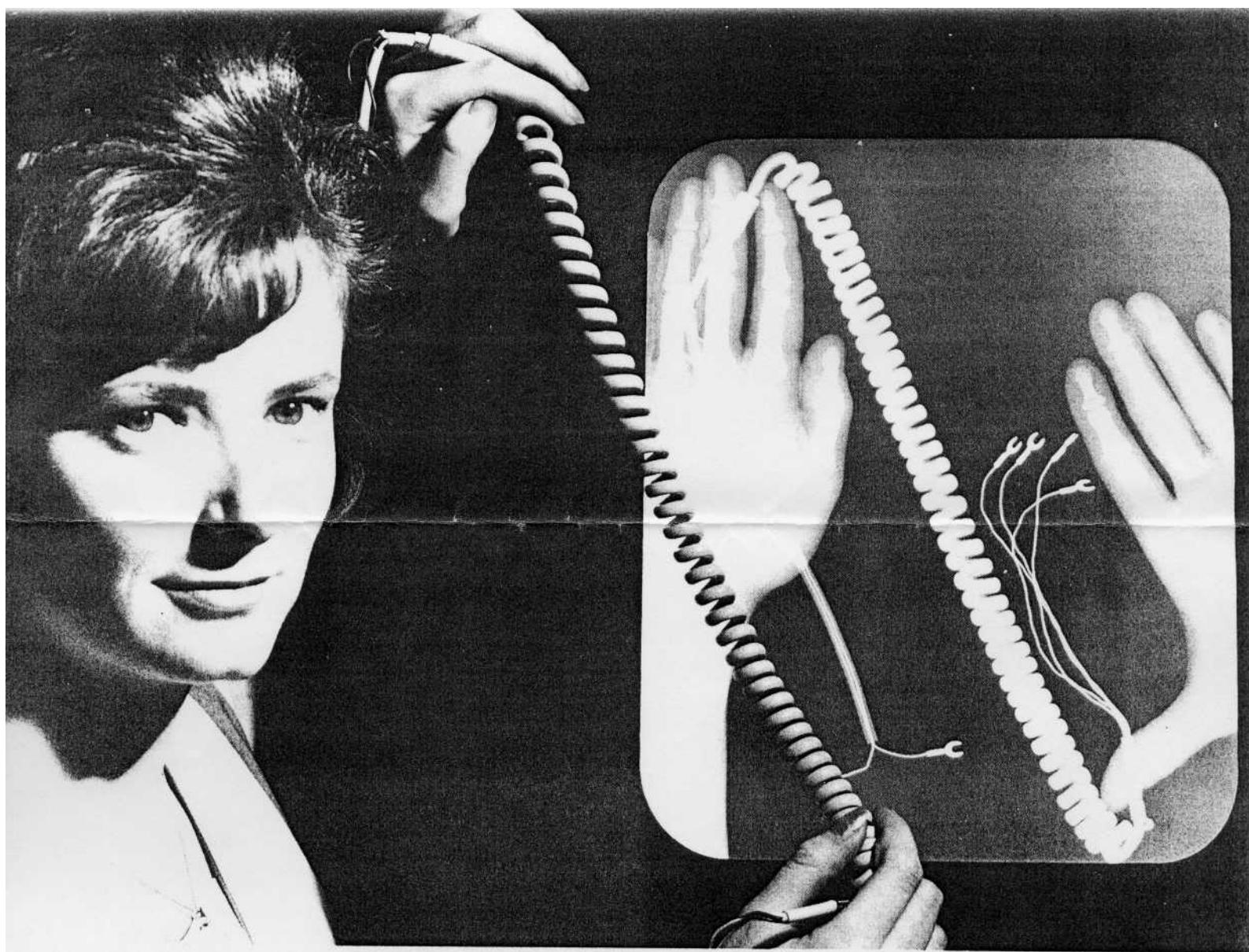
INSIDE STORY- WE's Carole Davison compares familiar telephone spring cord with an X-ray study of it. The X-ray shows the delicate winding of flexible bronze tinsel that runs beneath the plastic coating. E-212
