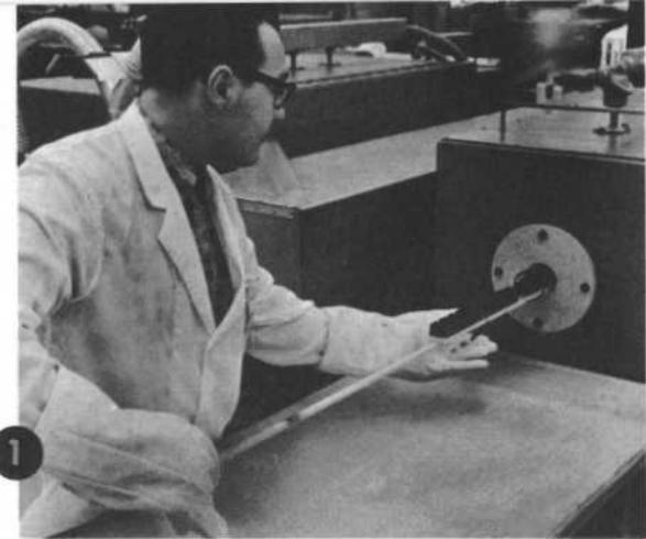
*Production of a solar cell starts with growing silicon crystals of the p (positive) type which are then sliced into thin strips. These strips go into a diffusion furnace where an n (negative) type material - such as phosphorus - is diffused into the surface of the strips. Where the electrical conductivity changes from n to p is the pn junction, the essential feature of a solar cell.*
