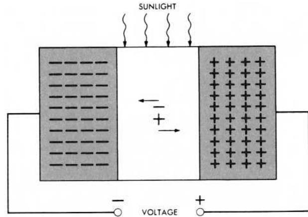
When internal photoemission takes place near a pn junction, the electric field forces conduction electrons energized by the light to go into the n-side, charging it negatively. Excess holes are similarly forced into the p-side, charging it positively. An electric circuit can use these charges in the same way that it uses the charge from a chemical battery. In this manner, silicon cells have converted as much as 12-15 per cent of the energy of incident sunlight directly into electricity.
