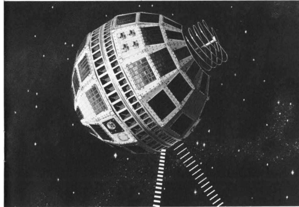
*All the power (13.5 watts) to operate the TELSTAR satellites comes from 3600 newly designed n-on-p solar cells mounted on the satellite's skin.*
