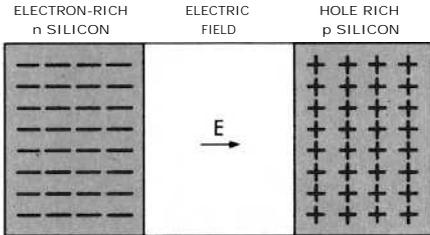
A semiconductor can have two kinds of movable electric charge, either negatively-charged "conduction electrons" (n-type) or positively-charged "holes" (p-type). If one region of a semiconductor is n-type while a neighboring region is p-type, there will be between them a strong electric field which tends to keep the positive holes in the p-side and the negative electrons in the n-side.
