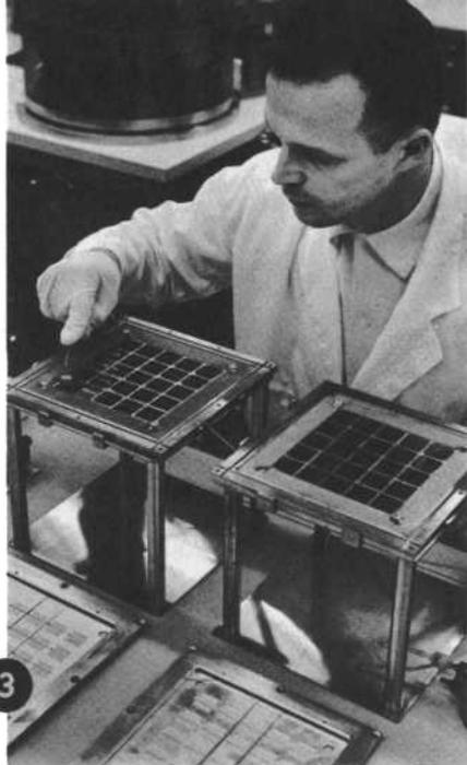
3 To make electrical contact to the n and p-layers so that power can be drawn from the cell, the slices are mounted in masks. Next, electrically conducting layers are deposited from the vapor state through the masks onto the crystals.
