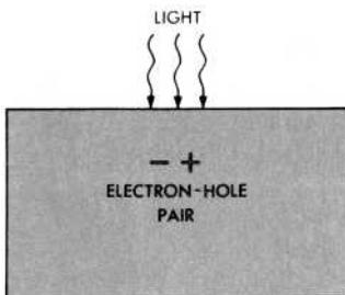
Light absorbed by a semiconductor breaks free some of the fixed or bound (nonconducting) electrons which hold the semiconductor together. When so energized, these electrons become "conduction electrons." They also leave behind in the binding structure "holes" which are positively-charged because the negative electrons are gone. This release of pairs of holes and electrons by the action of light is called "internal photoemission."
