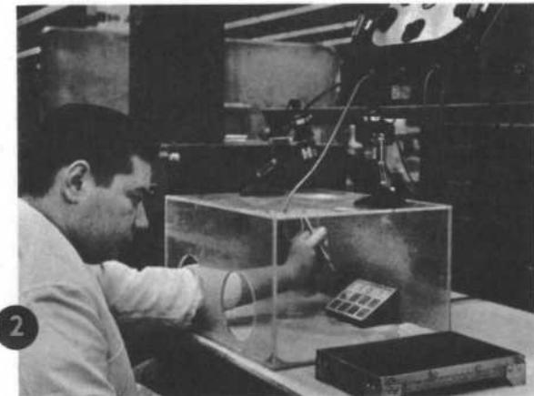
*As the diffused n-layer is required on only one surface of the slice - the surface facing the sun - it is removed from the other side by air blasting.*
