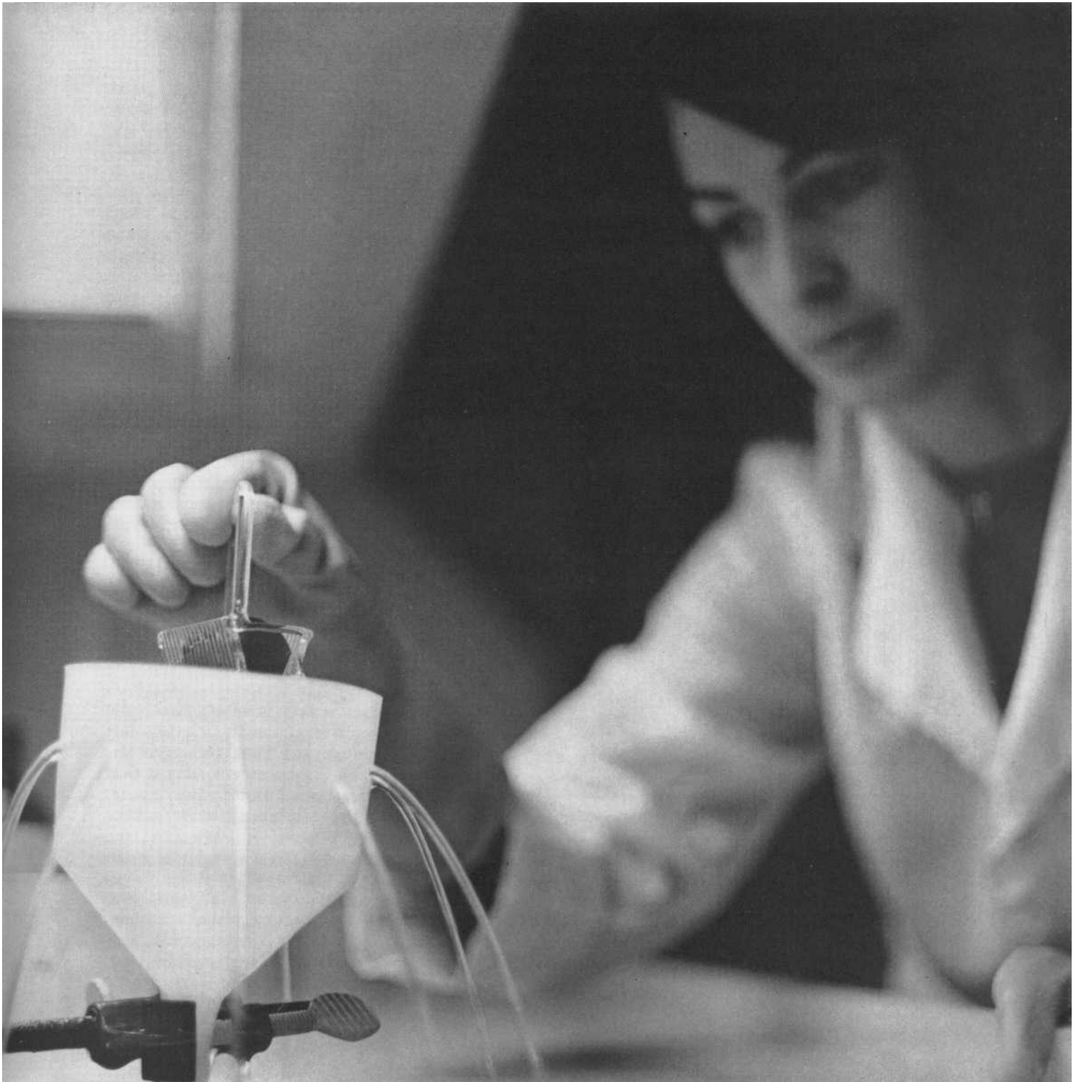
Miss Gloria Schirmacher of the Allentown Laboratory rinsing logic transistor slices in preparation for the diffusion process.
