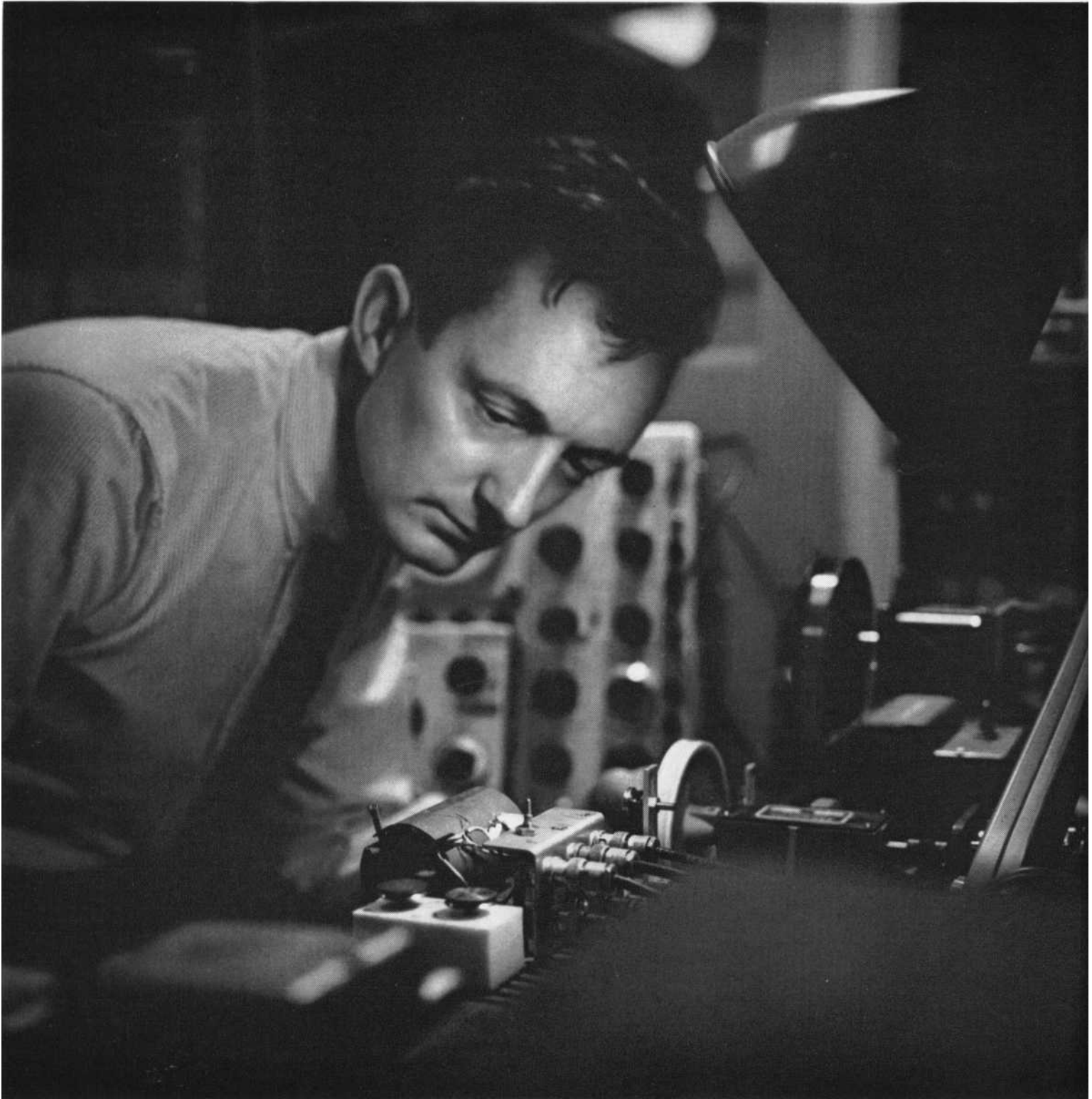
Continuous pulse testing is performed on all twistor wire for the permanent magnet twistor memory to ensure that the signal levels are uniform for binary one and binary zero readouts. L. L. Vanskike performs the test on wire to be fabricated into the device.
