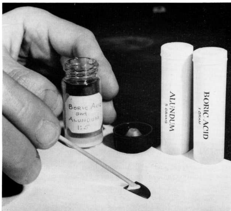
Figure 6-5. Painting the silicon slab with boric acid-Alundum-water mixture.
