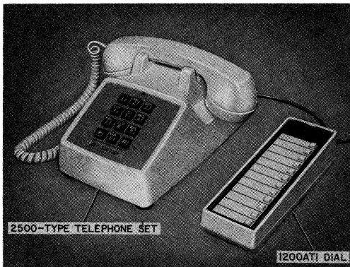
Fig. 2—1200AT1 Automatic Dialer and Associated TOUCH-TONE Service Telephone Set
