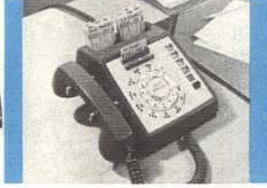
Integrated Card-Operated Dial telephone set designed to assist customers in dialing frequently called telephone numbers.
