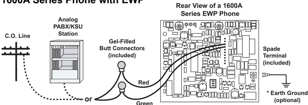
**\* Note:** *To increase surge protection, loosen the PCB mounting screw labeled ⊕ (as shown) and fasten a wire with spade terminal (included) from the mounting screw to Earth Ground (grounding rod, water pipe, etc.)*
