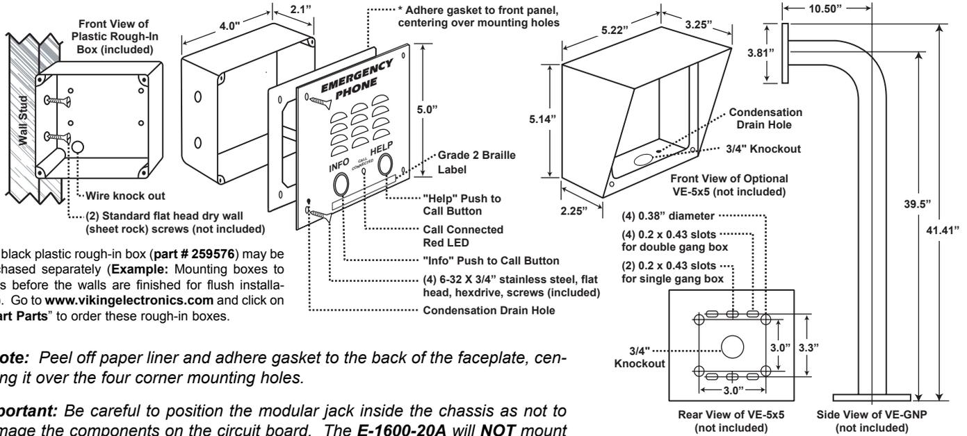
The black plastic rough-in box (part # 259576) may be purchased separately (Example: Mounting boxes to studs before the walls are finished for flush installation). Go to [www.vikingelectronics.com](http://www.vikingelectronics.com) and click on "Spart Parts" to order these rough-in boxes.
