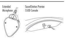
6. Plug the Power Adapter Cable into the 500D/550D Interface Module jack marked ⊕→⊕ then plug the Power Adapter into the electrical outlet.
