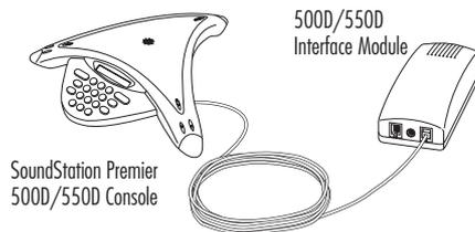
4. Plug the other end into the slot under the SoundStation Premier 500D/550D Console as illustrated.
