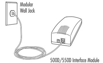
2. You have the option to install a DEFINITY series telephone along with your SoundStation Premier 500D/550D. Plug the DEFINITY Telephone cable into the jack on the 500D/550D Interface Module indicated by the telephone icon (
