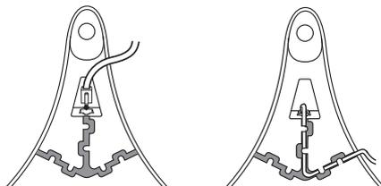
5. The SoundStation Premier 550D is designed for greater room coverage with extended microphones. If using the optional extended microphones, connect to SoundStation Premier 550D as shown at right.
