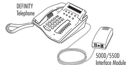
(If the connector does not fit you will need one of the optional cables as a replacement for your phone cable. This cable has a smaller connector on one end, so try it both ways.)
