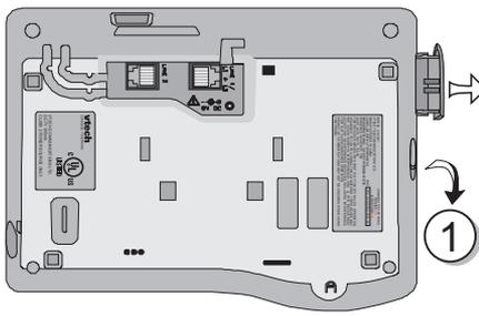
1. Open the spare battery charger by pressing the release button, located on the left-hand side of the Base Unit. A drawer will open to reveal the spare battery compartment.
