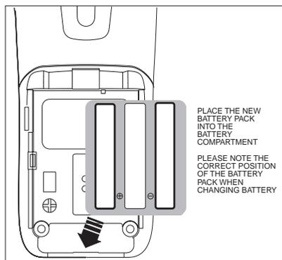
4. Replace the battery case cover by sliding the cover upwards.
