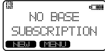
2. Press **NEW**, then enter the 15 digit Base Unit ID code, located on the underside of the Base Unit.
