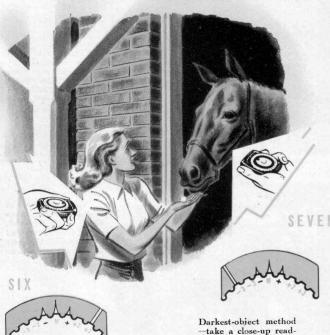
Darkest-object method—take a close-up reading of the darkest part of the subject that is in the shadow. This method is most useful when shadow detail must be included in an exposure for a scene of great brightness range.
