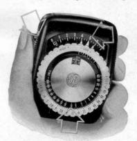
2 SET the trident in alignment with the meter pointer by turning the f-stop dial. See page 12. The light value is then automatically interpreted into exposure settings on the dials.
