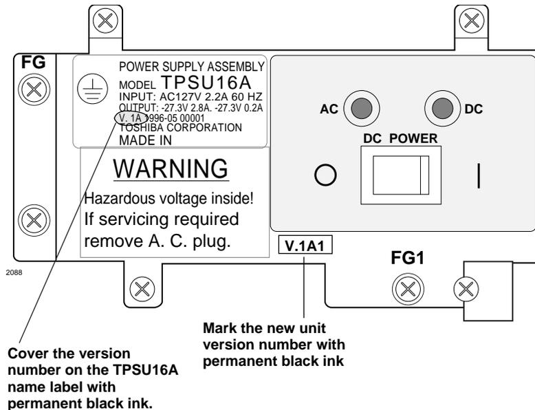
7. Insert the plug into the AC outlet. Turn on the DC power switch.
