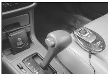
**From a portable CD player to your car stereo:** Connect the plug that is attached to the FM Transmitter to the Line Out or headphone jack of the CD player. Tune your car stereo to the transmitting frequency.
