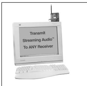
**From your computer to your home stereo:** Connect the plug that is attached to the FM Transmitter to the headphone jack on your speakers or to the audio output of the computer's sound card. Tune your receiver to the transmitting frequency.
