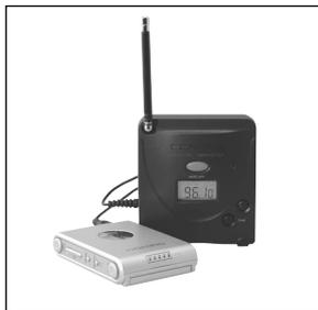
**From MP3 to a radio:** Connect the plug that is attached to the FM Transmitter to the Line Out or headphone jack of the MP3 player. Tune your radio or car stereo to the transmitting frequency.
