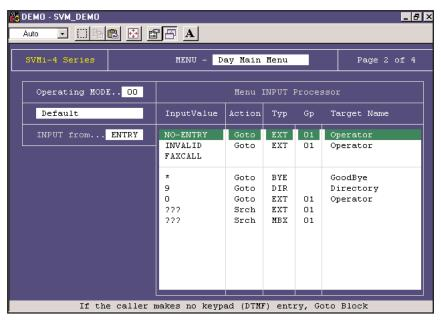
**Event Pointer** To make changes to the No-Entry, Invalid, and Faxcall Pointers, highlight the field and press ENTER to bring up the Target Generator. Highlight and open the appropriate Block type. Select a new or existing Block from the
