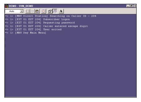
This screen provides the system administrator the ability to observe, port specific, line by line system activity in either real time (as it happens) or through
