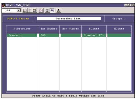
To view a subscribers data scroll to the correct subscriber using the arrow keys and press 'enter'. Use the right arrow key to select extension block or mailbox block. When you have made your selection press 'Ctrl + 0' (for open) and the
