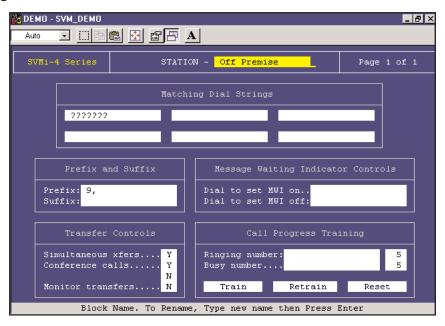
**Matching Dial Strings** This area is where the system matches the dialed digits. If a Station Block has not been explicitly assigned to a phone number SVMi-
