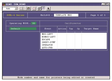
**Operating Mode** Indicates the Mode Name and Number for which the displayed Block Pointers' Targets are active. Operating Modes are given a unique Number by the system. In the SVMi-4 they are 01 - 04, indicating Day, Night, Holiday and Emergency / Bad weather.
