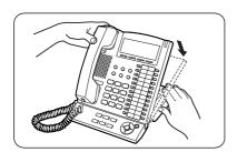
2 Connect the Ethernet cable, and then attach ① first and then ② of the wall mounting adaptor (included).
