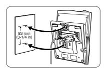
4 Pull down the handset hook until it locks, so the tab holds the handset.
