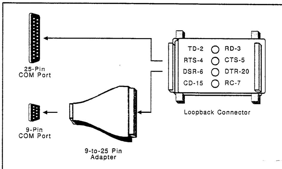
Figure 11 Loopback connector
