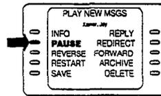
Options that may be set to ON or OFF may be “toggled” by pressing the soft key for that option. For example, if an option is set to ON, pressing the soft key sets it to OFF. In some cases, changing a setting from OFF to ON activates additional options on a display menu:
