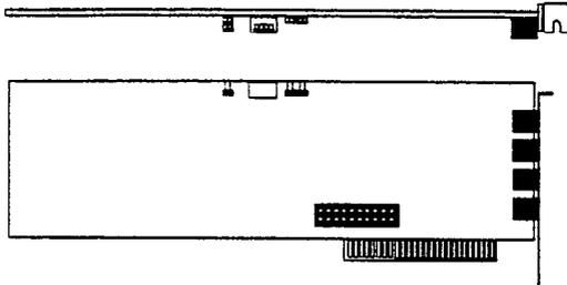
**Warning!** The voice board is easily damaged by static electricity.
