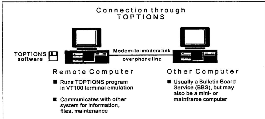
*Figure 33 Remote computer connected to BBS or other computer through TOPTIONS program*
