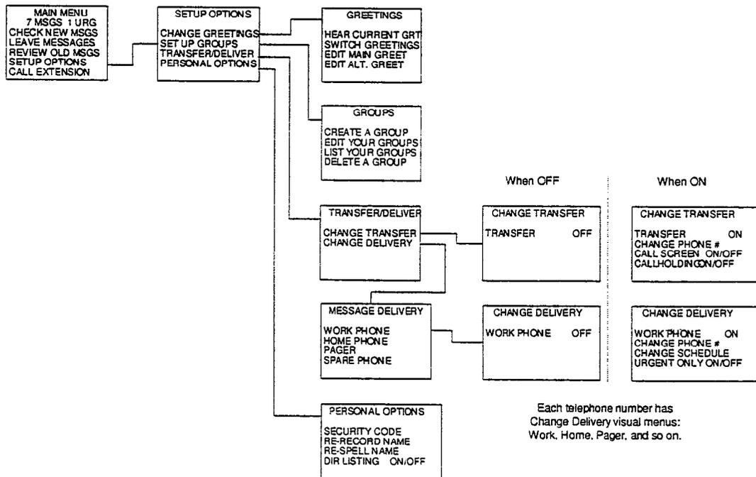
Figure 20 Visual menus used when accessing setup options using large-display phones
