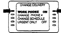
In addition to the soft keys on the Panasonic DBS large-display phone, the Integration Package supports additional keys located below the LCD. Note that these **fixed function keys** are labeled on the phone’s case, rather than on the LCD.
