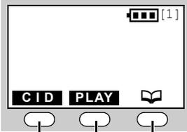
Three soft keys are used to select functions displayed directly above each key. Functions displayed above each key will change depending on the state of use.
