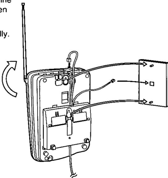
**5** Pull down the handset hook until it locks **so the tab holds the handset.**
