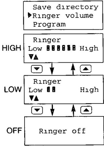
•When you replace the battery, the selected ringer volume setting will return to the factory set (HIGH). Reprogram if necessary.
