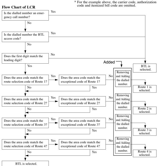
To activate this feature, please add the following new System Programming to the LCR Routing Plan Tables (Routes 1 through 4)
