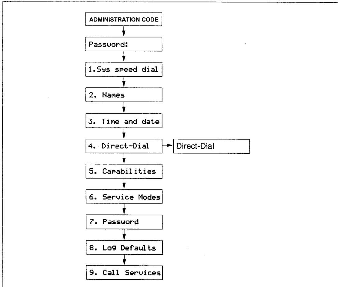
Use the  button, the **CHANGE** display button and the dial pad to enter the internal number of the telephone to be designated as the Direct-Dial telephone.
