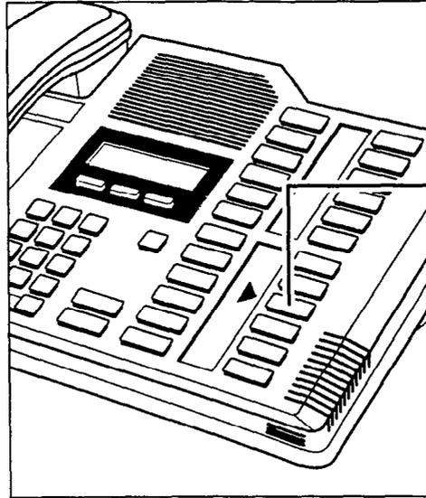
Memory buttons are the buttons with indicators other than line or Handsfree buttons. Memory buttons store telephone numbers or feature codes to give you one touch dialing or feature activation. You can change what a memory button does by just programming it with a new number or feature.
