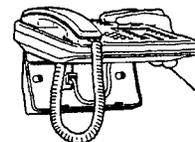
7. Connect the other end of the line cord to the wall jack. Store any spare cord neatly in the base of the telephone and mount the telephone on the base.
