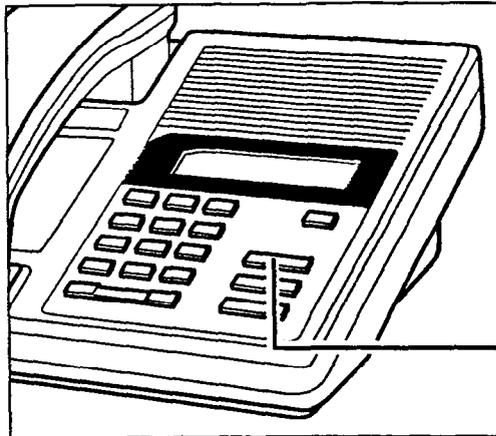
The memory button can store a telephone number or feature code to give you one touch dialing or feature activation. You can change the memory button by programming it with a new number or feature code.
