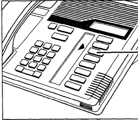
Memory buttons are the buttons with indicators other than line or Handsfree buttons. Memory buttons store telephone numbers or feature codes to give you one touch dialing or feature activation. You can change what a memory button does by just programming it with a new number or feature. You cannot program a line or Handsfree button.
