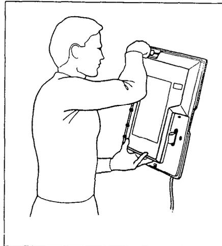
**Figure 2 — Inserting the Software Cartridge**
