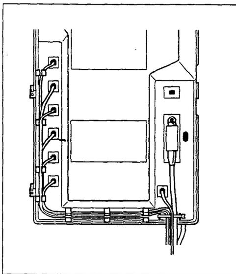
**Figure 4 — Plugging in the 25-pair cable**
