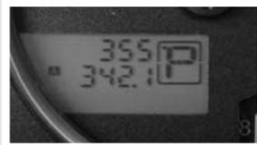
With the ignition key in the ON position or the vehicle running, you can select an item by pressing the CHANGE button on the instrument panel.
