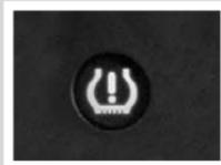
Tire pressure is affected by temperature. Low outside temperature causes lower tire pressure. This may cause the low tire pressure warning light to illuminate.
