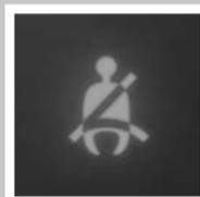
■ The seat belt warning light may also illuminate if the front passenger's seat belt is not fastened when the front passenger's seat is occupied. For 7 seconds after the ignition switch is in the ON position, the system does not activate the warning light for the front passenger.
