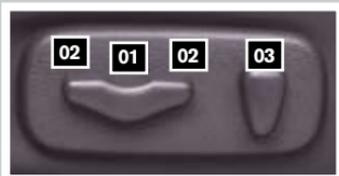
Your driver's seat has a lumbar support; adjust it by moving the lever up or down.
