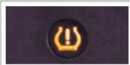
Tire pressure is affected by temperature. Low outside temperature causes lower tire pressure. This may cause the low tire pressure warning light to illuminate.
