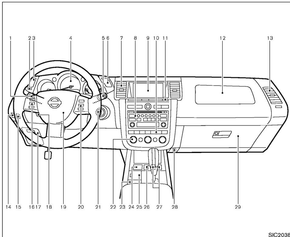
1. Headlight, fog light (if so equipped) and turn signal switch (P.2-19)
