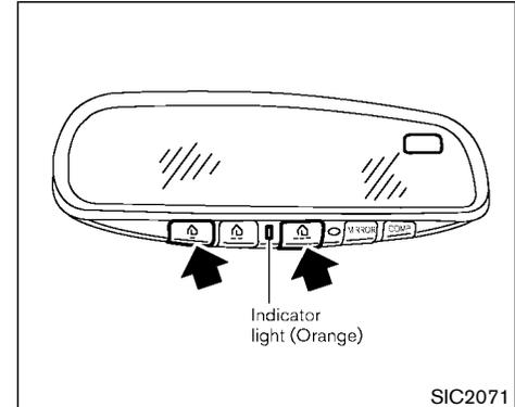
1. To begin, press and hold the 2 outer HomeLink® buttons (to clear the memory) until the indicator light blinks slowly (after 20 seconds). Release both buttons.
