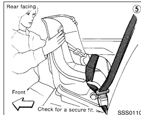
5. Before placing the child in the child restraint, use force to tilt the child restraint from side to side, and tug it forward to make sure that it is securely held in place.
