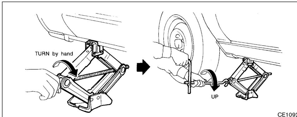
**The jack should be used on level firm ground.**
