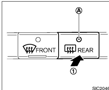
To defog/defrost the rear window glass and outside mirrors (if so equipped), start the engine and push the switch on ①. The indicator light ② will come on. Push the switch again to turn the defroster off.
