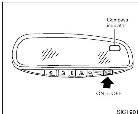
When the COMPASS switch is in the ON position, the compass display will indicate the direction the vehicle is heading.
