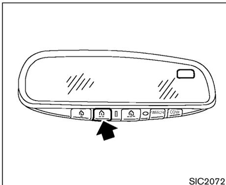
3. Using both hands, simultaneously press and hold both the HomeLink<sup>®</sup> button you want to program and the hand-held transmitter button.
