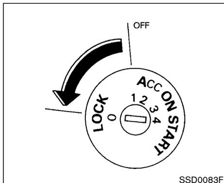
On CVT (Continuously Variable Transmission) models, the ignition lock is designed so that the key cannot be turned to LOCK and removed until the selector lever is moved to the P (Park) position.
