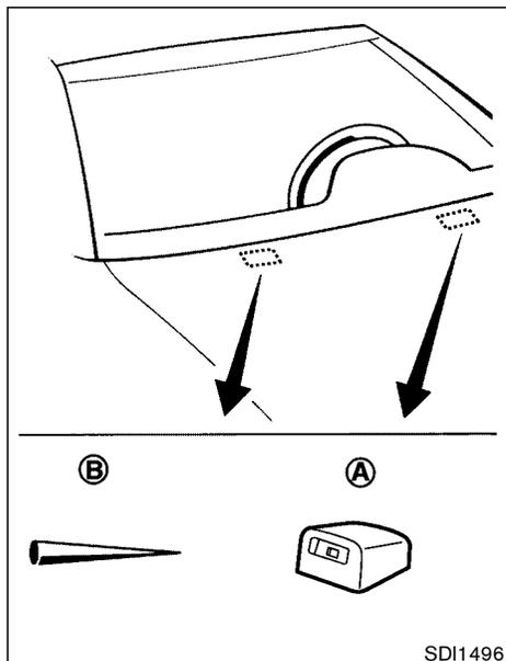
If you wax the surface of the hood, be careful not to let wax get into the washer nozzle. This may clog the nozzle (A) that could cause improper windshield washer operation. If wax gets into the nozzle, unclog it with a needle or small pin (B).
