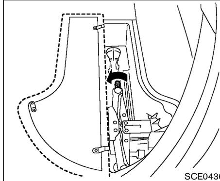
**Stowing the damaged tire and tools**
