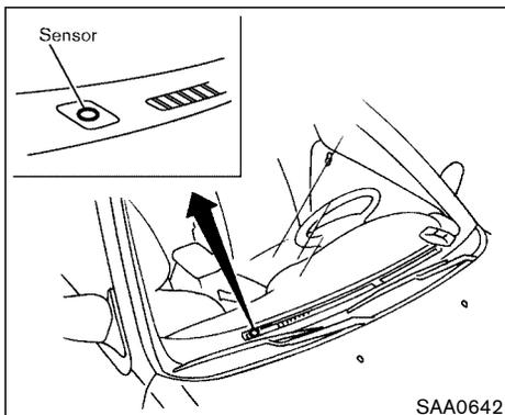
The sensor on the instrument panel helps maintain a constant temperature; do not put anything on or around this sensor.
