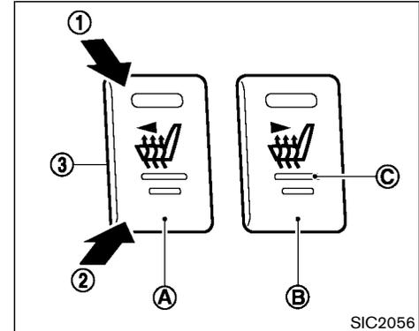
The front seats are warmed by built-in heaters. The switches located on the center console can be operated independently (driver side seat **A** and front passenger side seat **B**) of each other.
