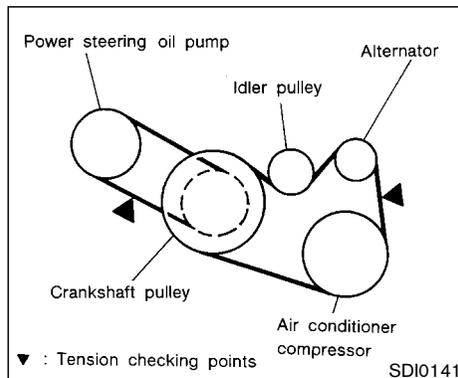
2. Have the belts checked regularly for condition and tension.
