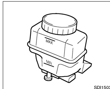
Check the fluid level in the reservoir. If the fluid is below the MIN line or the brake warning light comes on, add **DOT 3** fluid up to the MAX line. If fluid must be added frequently, the system should be thoroughly checked by your NISSAN dealer.
