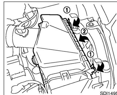
To remove the filter from the air cleaner, push down the lock pins ① and pull the unit upward ②.
