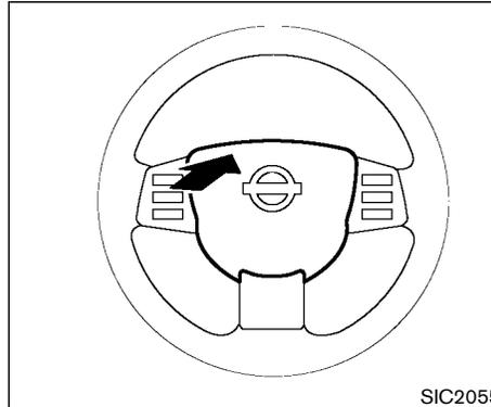
To sound the horn, push the center pad upper area of the steering wheel.
