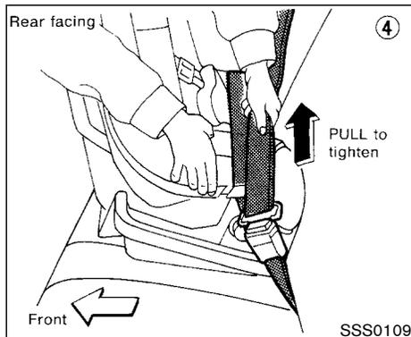
4. Allow the belt to retract. Pull up on the belt to remove any slack in the belt.
