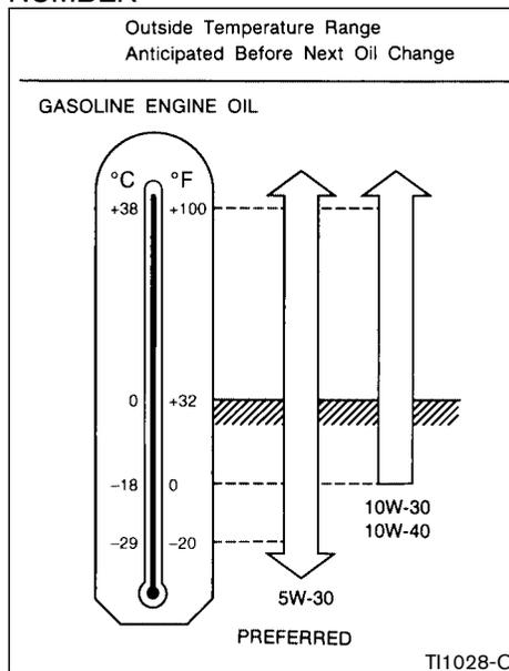
**SAE 5W-30 viscosity oil is preferred for all ambient temperatures. SAE 10W-30, 10W-40 viscosity oil may be used if the ambient temperature is above 0°F (-18°C).**
