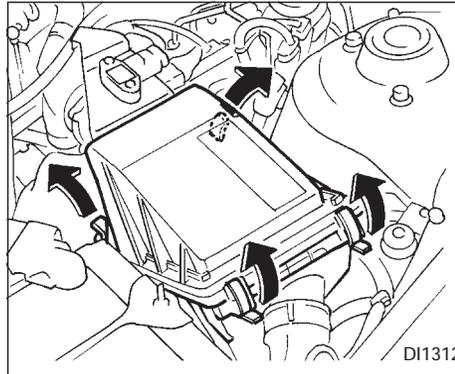
The air cleaner filter should not be cleaned and reused. Replace it according to the maintenance intervals shown in the “Maintenance schedule” section. When replacing the filter, wipe the inside of the air cleaner filter housing and the cover with a damp cloth.
