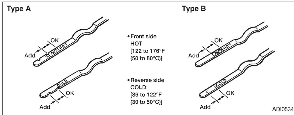
3. Check the fluid level with the engine idling.
