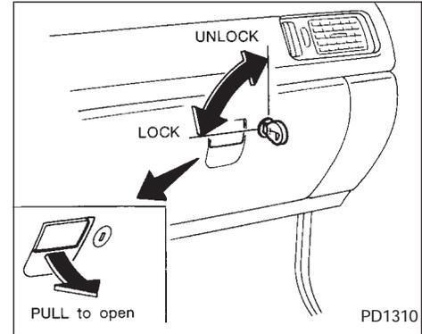
Use the master key to lock or unlock the glove box.
