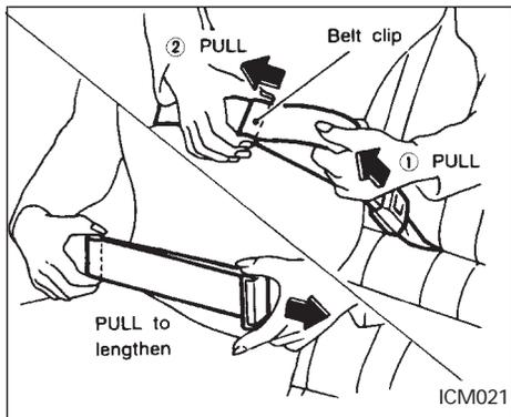
2. To lengthen, hold the tongue at a right angle to the belt and pull on the belt. To shorten, pull the end of the belt attached to the belt clip away from the tongue, then pull the belt clip to take up the slack.
