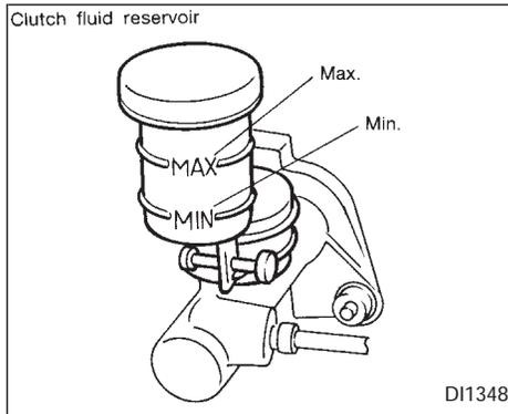
Check the clutch fluid level in the reservoir (manual transmission only). If the fluid level is below the MIN line, add **DOT 3** fluid up to the MAX line. If fluid must be added frequently, the system should be thoroughly checked by your NISSAN dealer.
