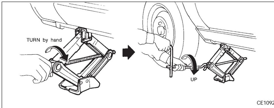
2. Loosen each wheel nut one or two turns by turning counterclockwise with the wheel nut wrench. **Do not remove the wheel nuts until the tire is off the ground.**
