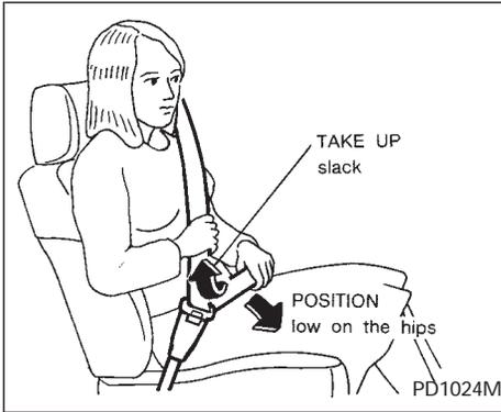
3. Position the lap belt portion **low and snug on the hips** as shown.
