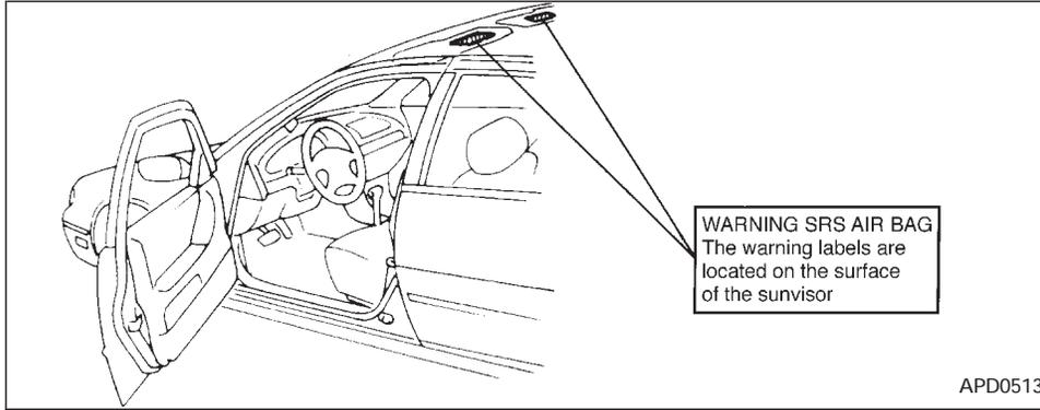
Warning labels about the supplemental air bag system are placed in the vehicle as shown in the illustration.
