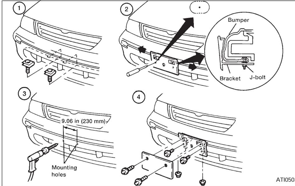
1. Insert J-bolts into the U-shaped grooves.
