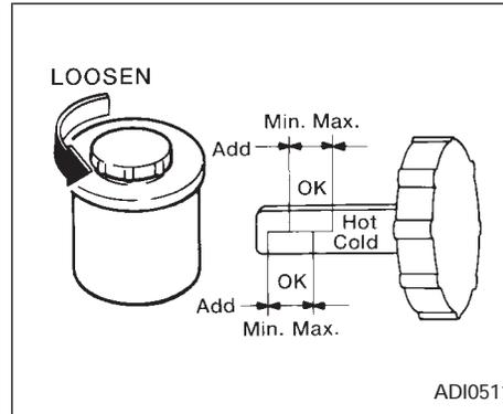
Check the fluid level in the reservoir.
