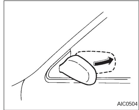
The driver and passenger outside mirrors are foldable. Push the outside mirror backward to fold it.
