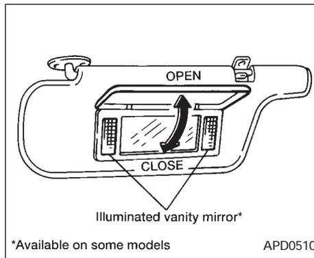
To access the vanity mirror, pull the sun visor down and flip open the mirror cover. Some vanity mirrors are illuminated and turn on when the mirror cover is opened.
