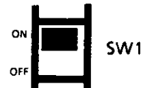
Figure 730-2 Battery Backup Switch SW1
