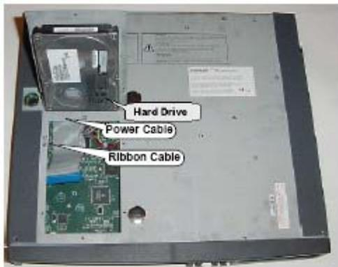
**Figure 18: LX and 700-User Controller Hard Drive Installation**
