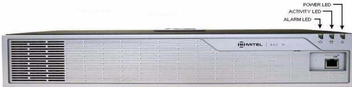
**Figure 98: ASU II LEDs**
