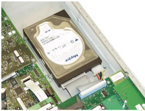
**Figure 19: MX Controller Hard Drive Installation**
