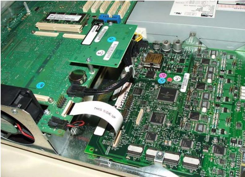
Figure 25: CX/CXi, AMB ribbon cable
