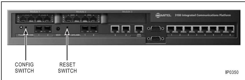
**Figure 14: CONFIG and RESET switches**
