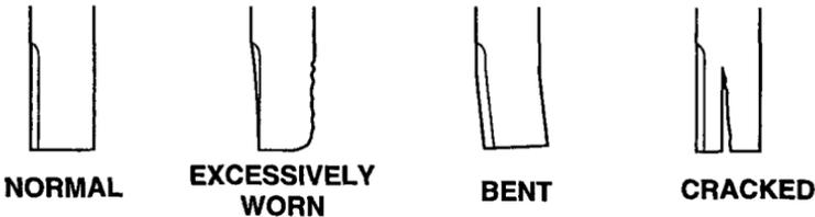
A dull blade can be sharpened, but a blade that is worn out, bent, cracked, or otherwise damaged must be replaced. A worn or damaged blade can break, causing blade pieces to be thrown from the mower.
