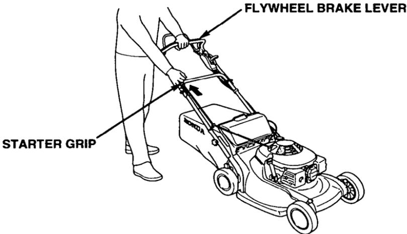
6. If the **CHOKE** position was used during starting, move the throttle lever away from the **CHOKE** position as soon as the engine warms up enough to run smoothly. Set the throttle lever at **FAST** to mow or at **SLOW** to idle.
