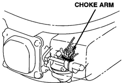
4. If the choke arm does not move all the way to its stop, in either direction, take the mower to an authorized Honda servicing dealer. Throttle cable adjustment involves related control plate adjustments.
