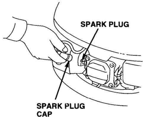
2. Remove the spark plug with a  $\frac{13}{16}$  in (21 mm) spark plug wrench.
