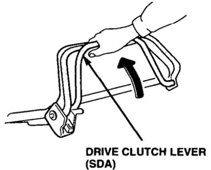
Operate the drive clutch lever with a quick and complete motion, so the drive clutch is either fully engaged or released. Hold the drive clutch lever against the handlebar during self-propelled mowing. This will help to extend the service life of the clutch mechanism.
