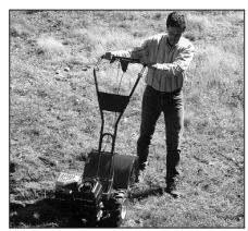
Fig. 4-5: With tines out of ground, push handlebars sideways to turn tiller.
