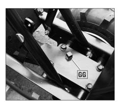
Fig. 2-11: Remove gear oil fill plug.
