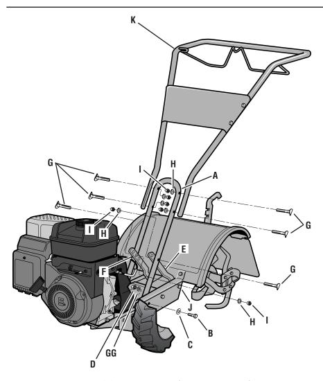
Fig. 2-2: Attach handlebar (5.5HP Model shown).
