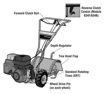
Figure 1-1: Tiller features and controls (5.5HP Model shown). See separate Engine Owner's Manual to identify engine controls.
