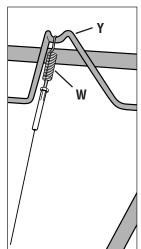
Fig. 2-6: Attach forward clutch cable spring to forward clutch bail.
