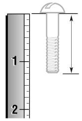
Figure 2-1: To identify length of screws, place screw on template as shown and measure distance between bottom of screw head and tip of screw.
