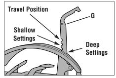
Figure 3-5: Depth Regulator Lever (G).
