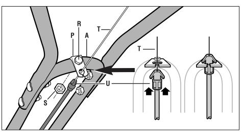
Fig. 2-4: Installing forward clutch cable bracket and cable.
