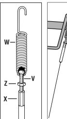
Fig. 2-5: Cable spring and adjuster.
