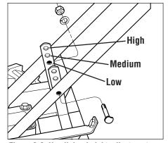
Figure 3-6: Handlebar height adjustment.
