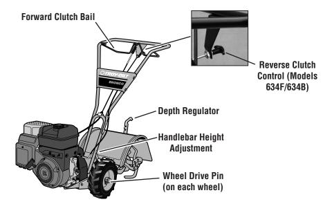
Figure 3-1: Tiller features and controls (5.5HP Model shown). See separate Engine Owner's Manual to identify engine controls.
