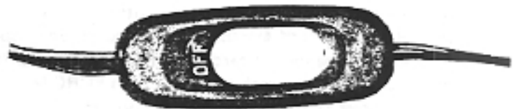
Figure 3.6.2.2.(2)(c) Switch on the PCRC-M
