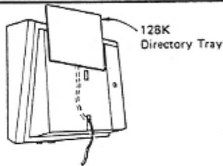
Figure 3.10.4.2(4)(h)A Modular Cord and 128K Pedestal Processing 1 (128K Directory Tray mounted in up position)
