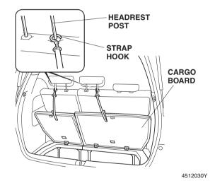
3. When you do not use the strap hook, secure it on the back side of the cargo board with a fastener.
