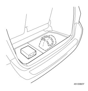
5. Cargo board can be used on either the right or left side only. Remove either right or left cargo board. Push the cargo board in the direction of the arrow and lower the seat slowly to store it.
