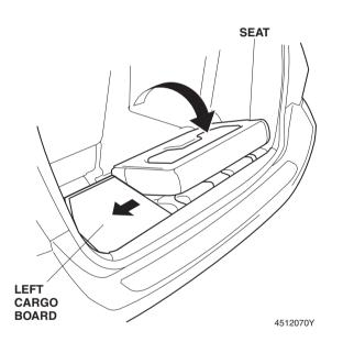
The maximum weight of the cargo board should no exceed 22 lbs (10 kg).
