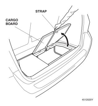
2. The cargo board can be held open by hooking the strap hook on the headrest post as shown. When the cargo board is held open with the strap hook, do not apply force to the cargo board such as by leaning against it.
