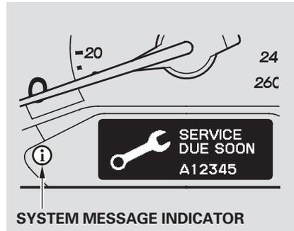
To see the current engine oil life, turn the ignition switch to the ON (II) position, then push and release the SEL/RESET button on the steering wheel repeatedly, until the engine oil life is displayed.
