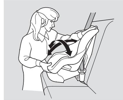
5. Push and pull the child seat forward and from side-to-side to verify that it is secure enough to stay upright during normal driving maneuvers. If the child seat is not secure, unlatch the belt, allow it to retract fully, then repeat these steps.
