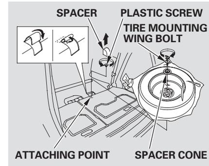
4. Place the flat tire face down on the attachment point. Put the spacer cone on the flat tire as shown. Poke holes in the vinyl bag. Secure the flat tire into the attachment point by tightening the tire mounting wing bolt through the center cap hole of the flat tire wheel.
