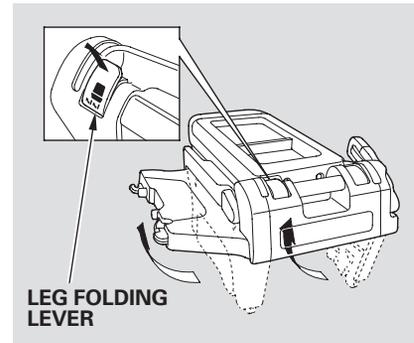
6. Fold the legs by pulling the leg folding lever.
