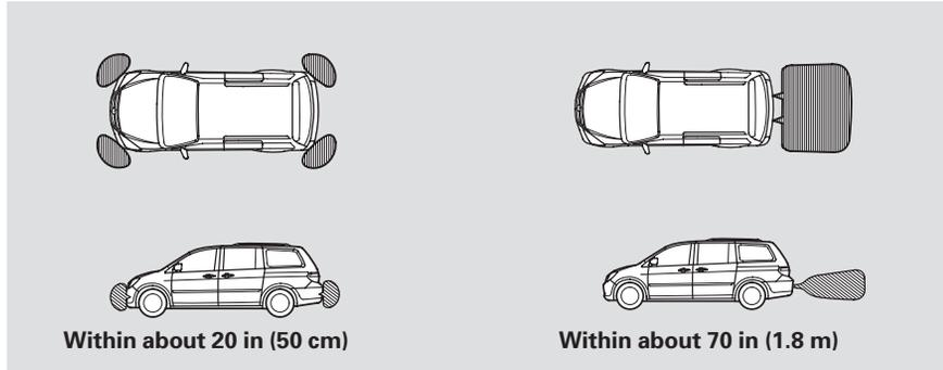
The range of the corner sensors and the rear center sensor are limited. Each corner sensor is capable of sensing an obstacle only when your vehicle is 20 in (50 cm) or closer. The rear center sensor senses an obstacle that is behind your vehicle 70 in (1.8 m) or closer.
