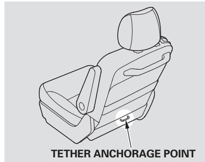
Each second row bucket seat has a tether anchorage point at the bottom of the seat-back.
