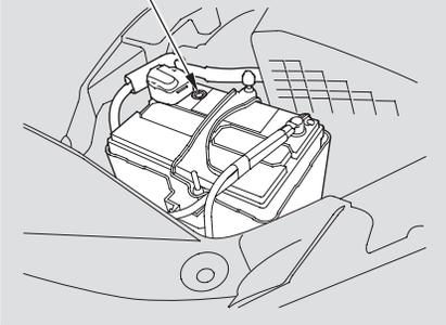
Check the condition of the battery monthly by looking at the test indicator window. The label on the battery explains the test indicator's colors.
