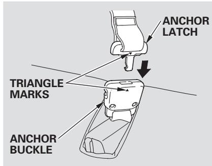
Insert the hook at the end of the anchor latch into the anchor buckle by lining up the triangle marks on the anchor latch and buckle. Make sure the belt is not twisted. Push the anchor latch until it locks. Then follow the procedure for fastening and positioning an ordinary seat belt (see page 15).
