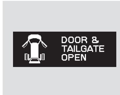
If the tailgate or any door(s) is not closed tightly, the display reminds you to close the tailgate or the door(s) before you start driving. This display continues until you close the door(s) or the tailgate. Pressing the INFO button on the steering wheel momentarily change the display to the normal display, but it will come back after 5 seconds.
