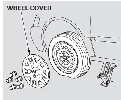
14. Remove the wheel nuts, then remove the flat tire. Handle the wheel nuts carefully; they may be hot from driving. Place the flat tire on the ground with the outside surface facing up.
