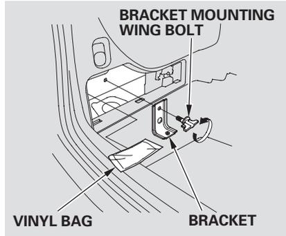
5. Remove the bracket from the jack storage area by unscrewing the bracket mounting wing bolt. Remove the vinyl storage bag.
