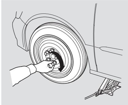
16. Put on the spare tire. Put the wheel nuts back on finger-tight, then tighten them in a crisscross pattern with the wheel nut wrench until the wheel is firmly against the hub. Do not try to tighten the wheel nuts fully.
