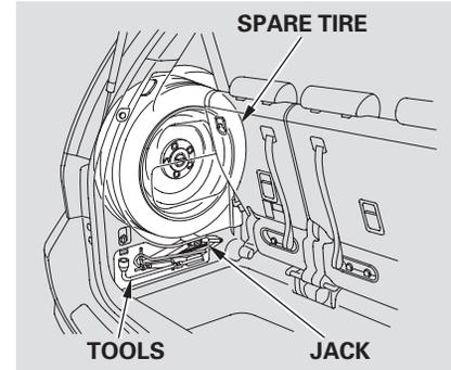
3. Open the tailgate. The jack is behind a cover in the cargo area on the driver's side, and tools are on the back of the cover. Remove the cover by pushing the tabs down and pulling the cover out.
