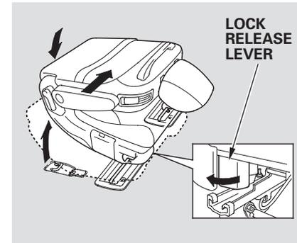
2. Unlock the seat from the floor by pulling the lock release lever under the seat cushion's front edge and lifting the rear of the seat.
