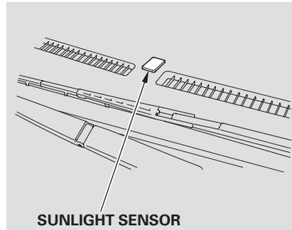
The climate control system has three sensors. A sunlight sensor is in the top of the dashboard, and a temperature sensor is next to the steering column. There is also a rear sensor on the rear sidewall near the exhaust vent. Do not cover the sensors or spill any liquid on them.
