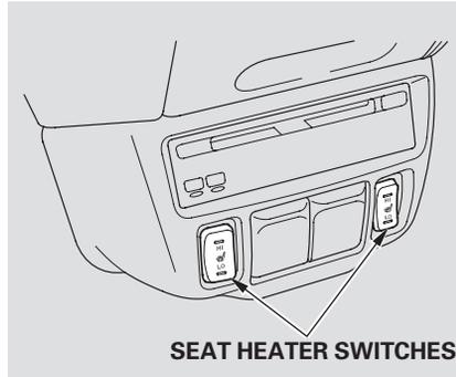
In HI, the heater turns off when the seat gets warm, and turns back on after the seat's temperature drops.
