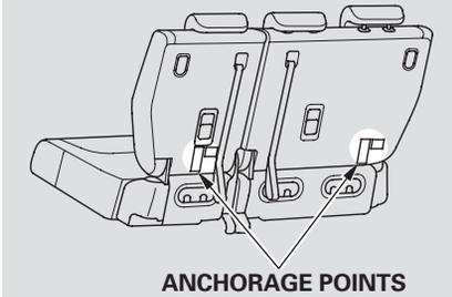
Each outside seating position of the third row has an anchorage point on the seat-back.
