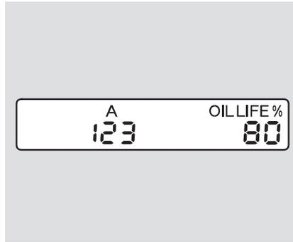
3. Press the Select/Reset knob for about 10 seconds. The engine oil life indicator and the maintenance item code(s) will blink.
