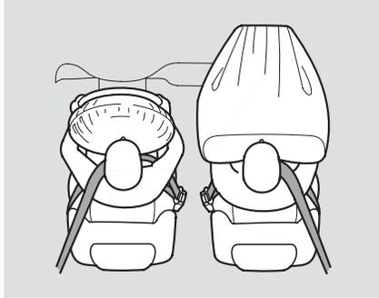
Your vehicle has a supplemental restraint system (SRS) with front airbags to help protect the heads and chests of the driver and a front seat passenger during a moderate to severe frontal collision (see page 27 for more information on how your front airbags work).
