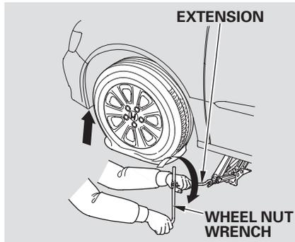
13. Use the extension and the wheel nut wrench as shown to raise the vehicle until the flat tire is off the ground.
