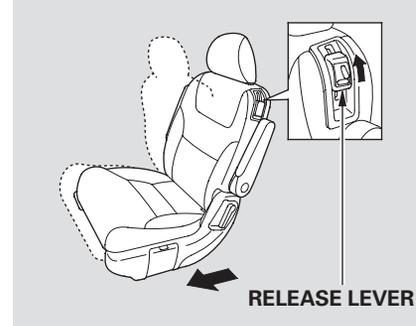
To get into or out of the third row seat, pull up the release lever on the shoulder of each second row bucket seat. The seat-back will tilt forward and the whole seat will slide forward.
