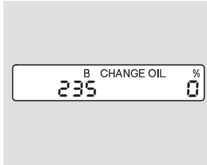
When the remaining engine oil life is 0 percent, you will see the above display. In this display, the remaining oil life indicator will be blinking. This display comes on and stays on every time you turn the ignition switch to the ON (II) position. When you see this message, have the indicated maintenance performed by your dealer as soon as possible.
