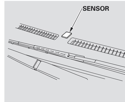
The automatic lighting feature is controlled by a sensor located on top of the dashboard. Do not cover this sensor or spill liquids on it.
