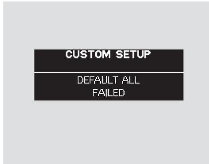
If “DEFAULT ALL” is not completed successfully, you will see the above display for several seconds, then the display goes back to the normal message mode. Repeat the procedure to select “DEFAULT ALL.”
