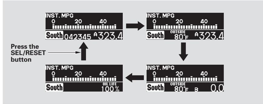
You can also change the display by pushing the select/reset knob in the instrument panel.
