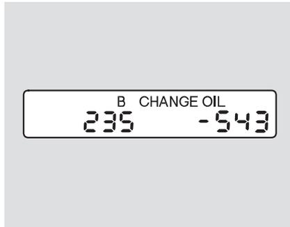
If you still do not perform the indicated maintenance, you will see a negative mileage, for example “-543,” blinking in the display. This negative mileage means that you should have performed the indicated maintenance 543 miles ago. Immediately have the indicated maintenance done by your dealer.
