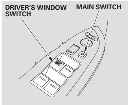
Turn the ignition switch to the ON (II) position to raise or lower any window. To open the window, push the switch down to the first detent and hold it. Release the switch when you want the window to stop. Pull back on the switch and hold it to close the window.
