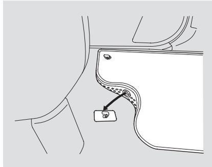
The driver's floor mat that came with your vehicle hooks over the floor mat anchors. This keeps the floor mat from sliding forward and possibly interfering with the pedals.
