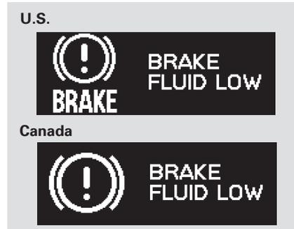
If the brake fluid level is at or below the MIN mark on the side of the brake fluid reservoir in the engine compartment, you will see “BRAKE FLUID LOW.” If you see this message, have the brake system checked by your dealer (see page 411).
