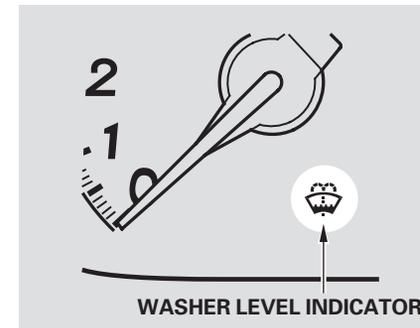
This indicator comes on when the washer fluid level is low. Add washer fluid when you see this indicator comes on (see page 366 ).
