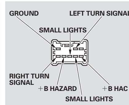
Your vehicle has a trailer lighting connector behind the right side panel in the cargo area. Refer to the drawing above for the purpose of each pin.
