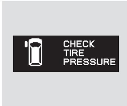
The TPMS monitors the air pressure of all four tires whenever the ignition switch is in the ON (II) position. It will immediately sense if a tire starts to lose its pressure, and give you warning with the low tire pressure indicator in the instrument panel and a “CHECK TIRE PRESSURE” message on the multi-information display. If the indicator and the warning message do not come on again after you inflate the tire to its correct air pressure (see page 384 ),
