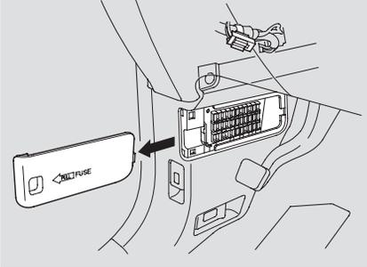
The vehicle's fuses are contained in four fuse boxes (three, if the vehicle does not have a rear entertainment system). The interior fuse boxes are located under the dashboard on the driver's and passenger's side.
