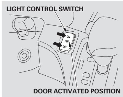
The light control switch controls the interior lights: the individual map lights in the front, the individual map lights above the second and third row passengers. This switch has three positions: OFF, door activated, and ON.
