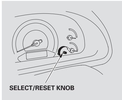
The Select/Reset knob on the instrument panel controls the brightness of the instrument panel lights. Turn the knob to adjust the brightness. Separate adjustments can be made when the headlights are on and off.
