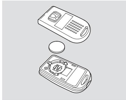
To replace the battery, separate the halves by carefully prying on the edge with a coin. Remove the old battery, and insert a new battery with the + side facing up. Snap the two halves of the transmitter case back together.
