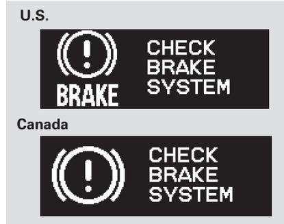
If there is a problem with the brake system, you will see “CHECK BRAKE SYSTEM” on the multi-information display. The parking brake and brake system indicator in the instrument panel will also come on. See page 411 for more information.
