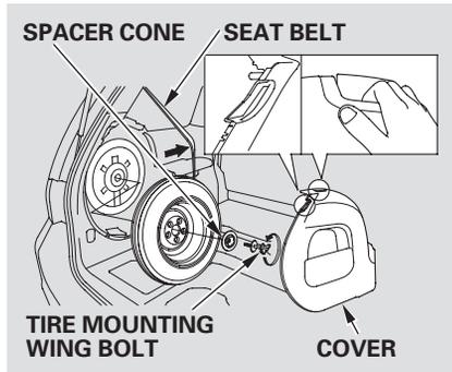
The spare tire is stored behind the spare tire cover on the sidewall of the cargo area on the driver's side.
