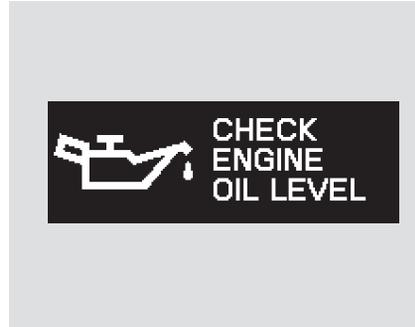
If the engine oil is very low or has lost pressure, you will see “CHECK ENGINE OIL LEVEL” on the multi-information display. You will also see the low oil pressure indicator in the instrument panel flashing or staying on. If you see this message, you should take immediate action since serious engine damage is possible. Follow the procedure on page 409 .
