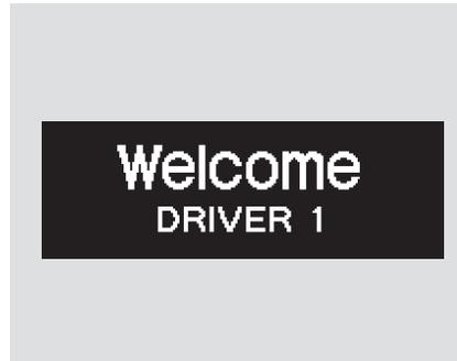
When you unlock and open the driver's door with the remote transmitter, the display shows "Welcome DRIVER 1" or "Welcome DRIVER 2" depending on which remote transmitter you use. The driver's "ID" is detected by the transmitter. For more information about driver's "ID", see page 152 .
