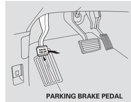
To apply the parking brake, push the pedal down with your foot. To release it, push on the pedal again. The parking brake indicator on the instrument panel should go out when the parking brake is fully released (see page 69).
