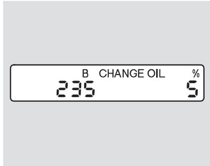
When the remaining engine oil life is less than 5 percent, you will see a “CHANGE OIL” message on the information display, along with the same maintenance item code(s), every time you turn the ignition switch to the ON (II) position.
