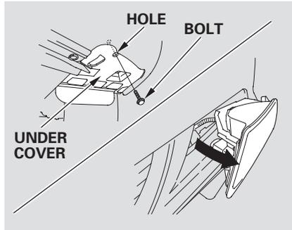
1. Remove the undercover bolt located under the front bumper.
