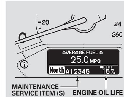
The multi-information display in the instrument panel shows you the engine oil life and maintenance service items when the ignition switch is in the ON (II) position. This information helps to keep you aware of the periodic maintenance your vehicle needs for continued trouble-free driving. Refer to page 347 for more information.
