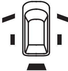
The appropriate light comes on in this monitor if the tailgate or any door is not closed tightly.
