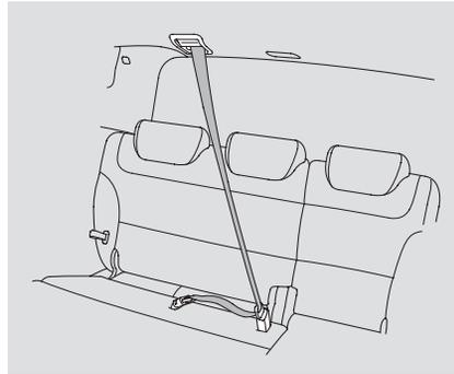
The lap/shoulder belt in the center seating position on the third seat and the stowable second row plus-one seat (depending on models) is equipped with a detachable anchor that has two parts: a small latch plate and an anchor buckle.
