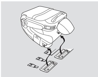
2. Unlock the seat from the floor by pulling the lock release lever under the seat cushion's front edge and lifting the rear of the seat.
