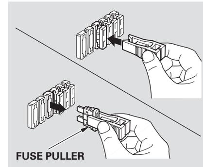
4. Check the smaller fuses in the under-hood fuse box and all the fuses in the interior fuse boxes by pulling out each fuse with the fuse puller provided in the primary under-hood fuse box.
