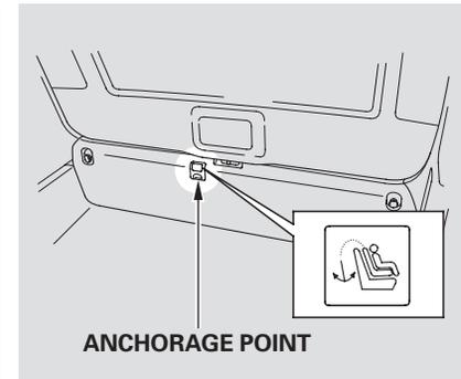
The center seating position of the third row has an anchorage point on the tailgate sill.
