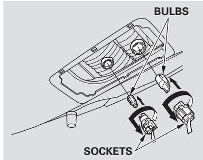
3. Remove the socket by turning it one-quarter turn counterclockwise.
