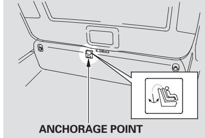
The center seating position of the third row has an anchorage point on the tailgate sill.
