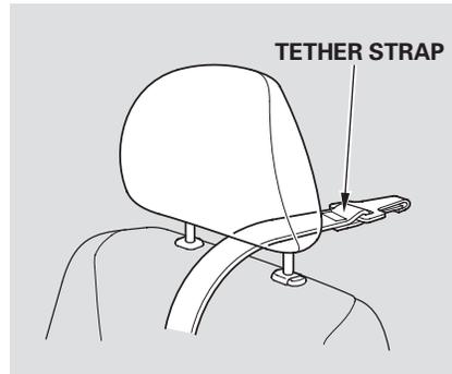
5. Lift the head restraint (see page 174 ), then route the tether strap through the legs of the head restraint, over the seat-back and through the grab rail.
