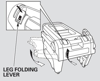
To install the stowable plus-one seat, extend the legs by pulling the leg folding lever.
