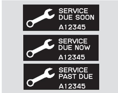
When the engine oil life reaches 15 %, the display shows “SERVICE DUE SOON” and the code for the maintenance items to be performed.
