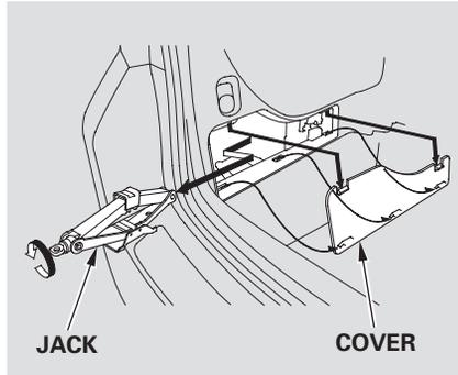
4. Loosen the jack from its holder by turning the end counterclockwise.
