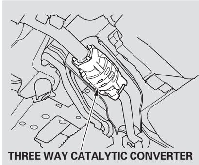
A defective three way catalytic converter contributes to air pollution, and can impair your engine's performance. Follow these guidelines to protect your vehicle's three way catalytic converter.
