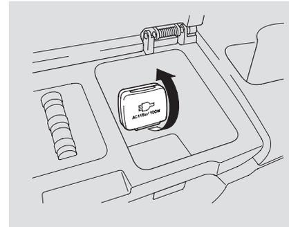
There is a 115 volt AC power outlet in the rear compartment on the driver's side. To use the AC power outlet, open the rear compartment lid and open the outlet cover. Insert the plug into the receptacle slightly, turn it 90° clockwise, then push in the plug all the way.
