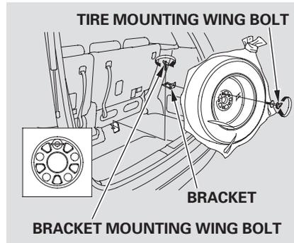
22. Install the bracket and the bracket mounting wing bolt on the attachment point as shown, and tighten the bolt. Make sure the bracket is securely tightened.
