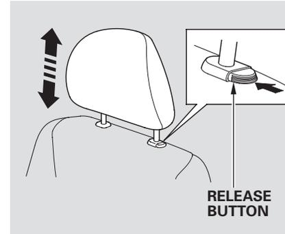
All head restraints adjust for height. You need both hands to adjust the restraint. Do not attempt to adjust it while driving. To raise it, pull upward. To lower the restraint, push the release button sideways, and push the restraint down.
