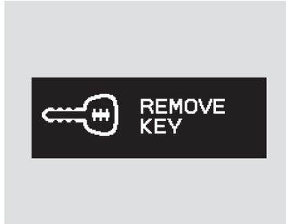
If you leave the key in the ignition switch in the LOCK (0) or ACCESSORY (I) position and open the driver's door, you will see "REMOVE KEY" on the display and hear a reminder beeper.
