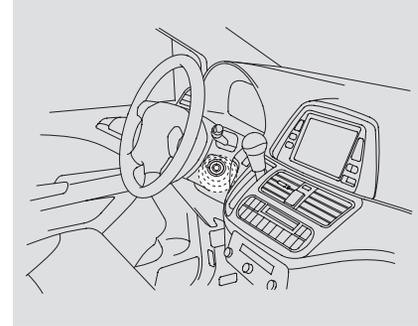
The ignition switch light comes on when you open the driver's door, and stays on several seconds after you close the door.
