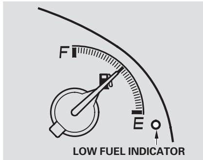
This indicator is in the fuel gauge. It comes on as a reminder that you must refuel soon. When the indicator comes on, there is about 3.01 US gal (11.4 ℓ) of fuel remaining in the tank before the reading reaches E. There is a small reserve of fuel remaining in the tank when the reading does reach E.
