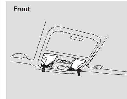
Turn on the front and rear individual map lights by pushing the lens of each light. Push the lens again to turn it off. You can also operate these lights with the light control switch (see page 208).
