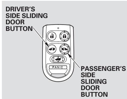
You can open or close each sliding door with the remote transmitter when the doors are unlocked. Push and hold the right button to open or close the passenger's side door, and the left button to open or close the driver's side door.
