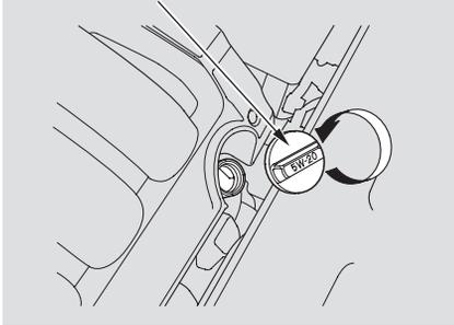
Unscrew and remove the engine oil fill cap on top of the valve cover. Pour in the oil slowly and carefully so you do not spill. Clean up any spills immediately. Spilled oil could damage components in the engine compartment.
