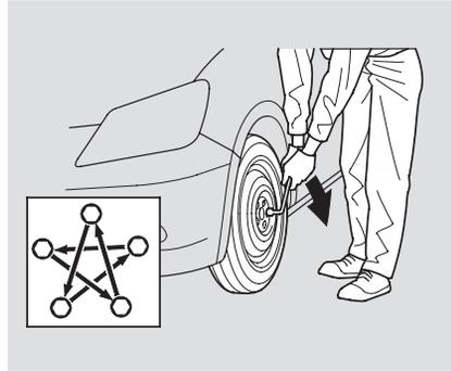
18. Tighten the wheel nuts securely in a crisscross pattern. Have the wheel nut torque checked at the nearest automotive service facility. Tighten the wheel nuts to:
