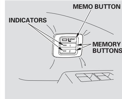
3. Press and release the MEMO button on the driver's door. You will hear a beep. Then, both indicators in the memory buttons will start to blink. Press and hold one of the memory buttons (1 or 2) within 5 seconds after you press the MEMO button. When the system completes storing a new driving position, you hear two beeps. The indicator in the stored memory button will come on.
