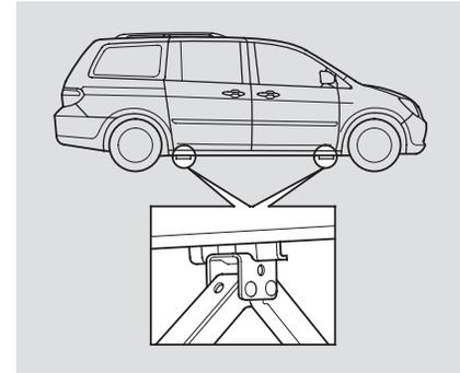
12. Place the jack under the jacking point nearest the tire you need to change. Turn the end bracket clockwise until the top of the jack contacts the jacking point. Make sure the jacking point tab is resting in the jack notch.
