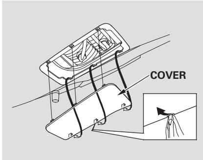
1. Open the tailgate. Place a cloth on the edge of the light assembly cover. Remove the cover by carefully prying in the notch on its middle edge with a flat-tip screwdriver.
