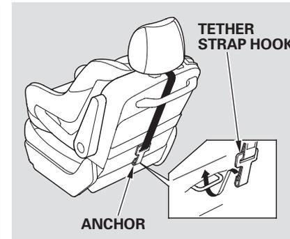
6. Attach the tether strap hook to the anchor, making sure the strap is not twisted, then tighten the strap according to the seat maker's instructions.
