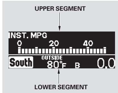
The multi-information display consists of two segments; an upper segment and a lower segment.
