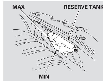
Look at the coolant level in the radiator reserve tank. Make sure it is between the MAX and MIN lines. If it is below the MIN line, see **Adding Engine Coolant** on page 364 for information on adding the proper coolant.
