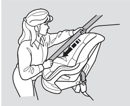
2. To activate the lockable retractor, slowly pull the shoulder part of the belt all the way out until it stops, then let the belt feed back into the retractor.
