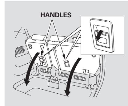
3. Pull the handle on each seat-back to unlock the front legs of the third seat.
