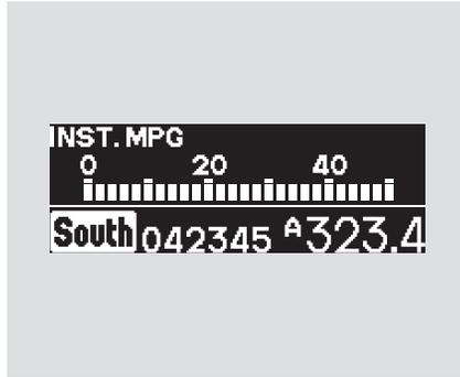
In the lower segment, each time you press the SEL/RESET button on the steering wheel, the display changes from “Trip A/Odometer” to “Trip A/Outside Temperature” to “Trip B/Outside Temperature” to “Engine Oil Life”, and then back to the “Trip A/Odometer” as shown in the next column.
