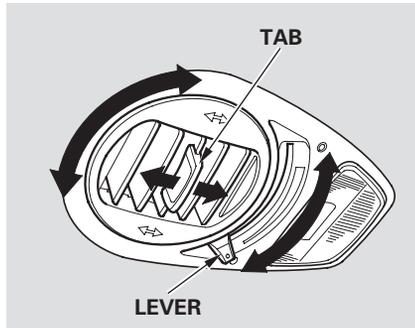
The direction and quantity of airflow from each rear ceiling vent is adjustable.
