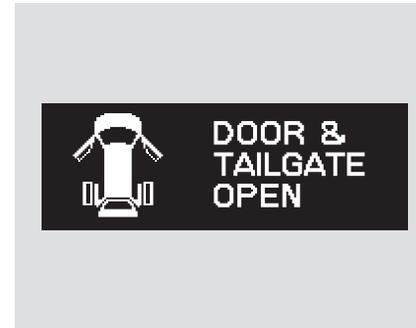
The door and tailgate open monitor appears on the multi-information display to indicate when a specific door or the tailgate is not tightly closed.
