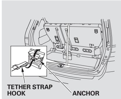
4. Remove the head restraint (see page 174). Make sure the removed head restraint is secured in the cargo area. Reinstall the head restraint when the child seat is removed.
