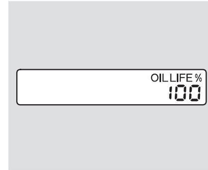
4. Press the Select/Reset knob for more than 5 seconds. The maintenance items code(s) will disappear, and the engine oil life indicator will reset to "100."
