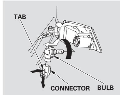
4. Remove the electrical connector from the bulb by pushing on the tab and pulling the connector down.
