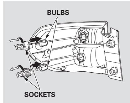
3. Determine which of the two bulbs is burned out: turn signal or brake/taillight.
