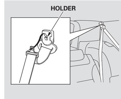
6. Move the seat belt out of the way by hanging the latch plate on the holder.
