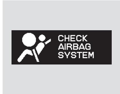
If there is a problem with your front airbags, side airbags, passenger’s side airbag automatic cutoff system, automatic seat belt tensioners, side curtain airbags, driver’s seat position sensor, or the front passenger’s weight sensors, you will see “CHECK AIRBAG SYSTEM” on the multi-information display. Take your vehicle to a dealer as soon as possible (see page 34).
