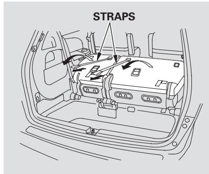
2. Pull the seat-back upright with the strap. Make sure the seat is securely locked into position before driving.
