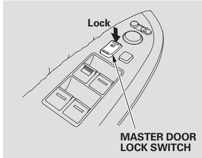
To lock the doors and the tailgate, press the front of the master door lock switch on either front door, press the lock tab on the driver's door, or use the outside lock on the driver's door.
