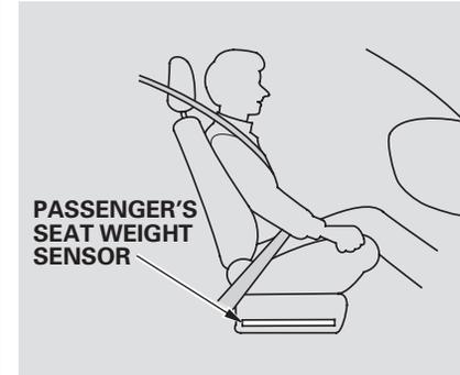
The passenger's advanced front airbag system has weight sensors under the seat. Although Honda does not encourage carrying an infant or small child in front, if the sensors detect the weight of an infant or small child (up to about 65 lbs or 29 kg), the system will automatically turn the passenger's front airbag off.
