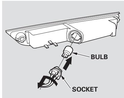
3. Remove the socket from the light assembly by turning it one-quarter turn counterclockwise.
