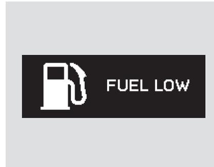
If the level of the fuel in the tank gets low, you will see “FUEL LOW” on the multi-information display, and you must refuel soon. The low fuel indicator on the instrument panel will also come on.
