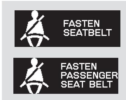
In addition to the seat belt reminder indicator on the instrument panel, the multi-information display interrupts the current display and shows “FASTEN SEAT BELT” or “FASTEN PASSENGER SEAT BELT” if you or your front passenger do not fasten your seat belts while driving. This message remains displayed if you ignore it and do not wear your seat belts while the vehicle is moving.
