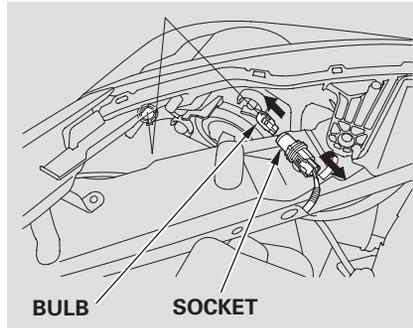
1. Open the hood. Remove the socket from the headlight assembly by turning it one-quarter turn counterclockwise.
