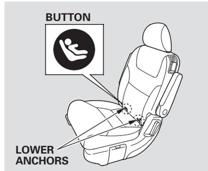
To install a LATCH-compatible child seat in a second row seat:
