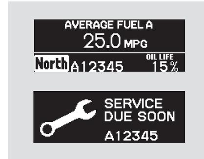
When the remaining engine oil life is 15 percent or less, the display shows a “SERVICE DUE SOON” message along with the maintenance item code(s) for other scheduled maintenance items needing service.
