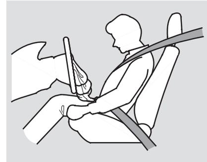
After inflating, the front airbags will immediately deflate, so they won't interfere with the driver's visibility, or the ability to steer or operate other controls.
