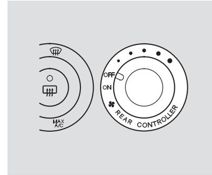
**ON** – With the dial in this position, the rear control panel can be used by a second row passenger to adjust the rear fan speed, airflow, and temperature.
