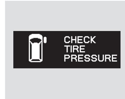
When any of the tires have low pressure, the low tire pressure indicator on the instrument panel comes on, and the multi-information display also interrupts the current display and shows a "CHECK TIRE PRESSURE" message. You can see one or more of the low pressure tire positions highlighted in the display along with this message.
