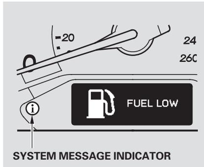
The system message(s) triggers the appropriate indicator(s) on the instrument panel, including the system message indicator, to come on. The system message indicator does not go off until the problem(s) is corrected.
