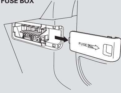
To open the passenger's fuse box, pull the right edge of the cover.
