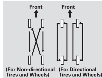
To help increase tire life and distribute wear more evenly, rotate the tires according to the maintenance messages displayed on the information display or multi-information display (depending on models). Move the tires to the positions shown in the diagram each time they are rotated. If you purchase directional tires, rotate only front-to-back.
