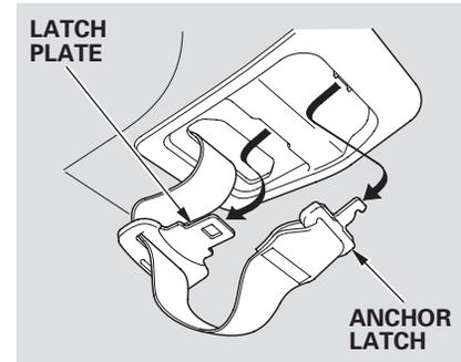
The plus-one seat on EX and EX-L models that can be installed in the center seating position of the second row also has a detachable seat belt anchor.
