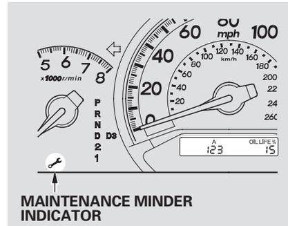
To see the current engine oil life, turn the ignition switch to ON (II), and push and release the Select/Reset knob on the instrument panel repeatedly, until the engine oil life is displayed.
