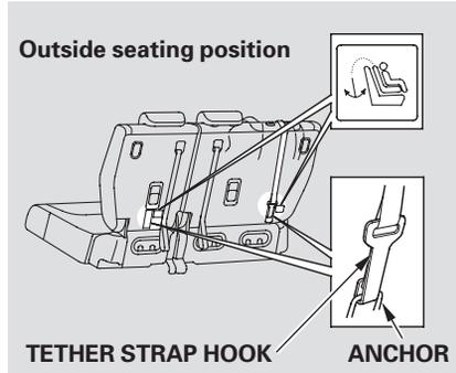
4. Attach the tether strap hook to the anchor, making sure the tether strap is not twisted.
