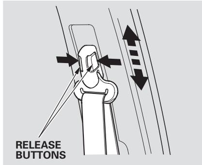
The front seats and second row seats have adjustable seat belt anchors. To adjust the height of an anchor, squeeze the two release buttons, and slide the anchor up or down as needed (it has four positions).
