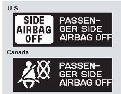
If the passenger's side airbag has automatically shut off, you will see "PASSENGER SIDE AIRBAG OFF" on the multi-information display. See page 35 for more information.
