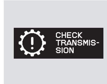
If there is a problem with the automatic transmission, you will see “CHECK TRANSMISSION” on the multi-information display. Avoid rapid acceleration, and have the transmission checked by a dealer as soon as possible.
