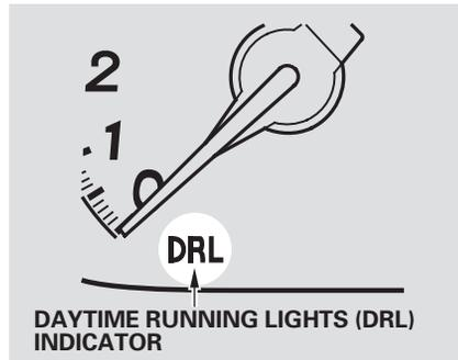
If this indicator comes on when the ignition switch is turned to the ON (II) position and the parking brake is released, it means there is a problem in the high beam headlight's circuit. Have your vehicle checked by your dealer.
