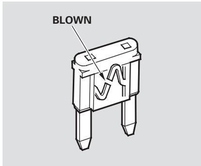
5. Look for a blown wire inside the fuse. If it is blown, replace the fuse with one of the spare fuses of the same rating or lower.
