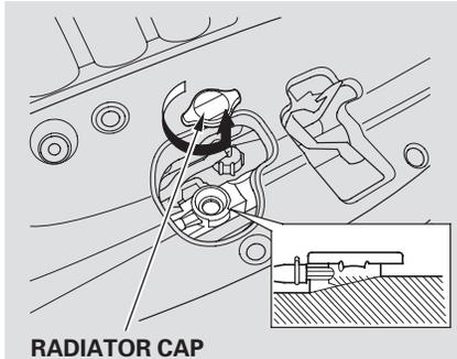
1. When the radiator and engine are cool, relieve any pressure in the cooling system by turning the radiator cap counterclockwise, without pressing down.
