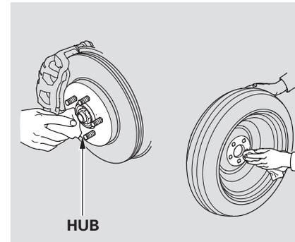
15. Before mounting the spare tire, wipe any dirt off the mounting surface of the wheel and hub with a clean cloth. Wipe the hub carefully; it may be hot from driving.
