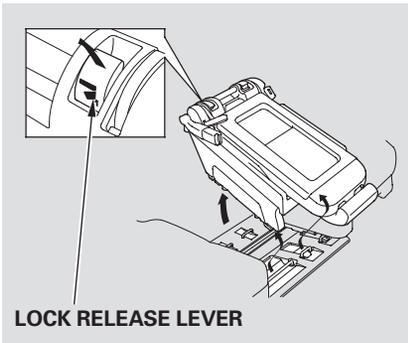
4. Unlock the seat from the floor by pulling the lock release lever and lifting the rear of the seat.
