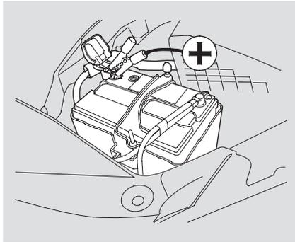
3. Connect one jumper cable to the positive (+) terminal on your vehicle's battery. Connect the other end to the positive (+) terminal on the booster battery.
