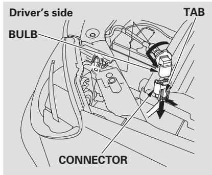
2. Remove the electrical connector from the bulb by pushing on the tab and pulling the connector down.
