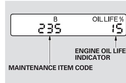
If the oil life is 15 percent or less, you will see the oil life indicator for every time you turn the ignition switch to the ON (II) position. This indicator stays on until you cancel it by pressing the Select/Reset knob. The maintenance minder indicator will also come on, and the maintenance item code(s) for other scheduled maintenance items needing service will be displayed next to the engine oil life indicator.
