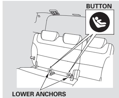
The location of each lower anchor is indicated by a small button above the anchor point.
