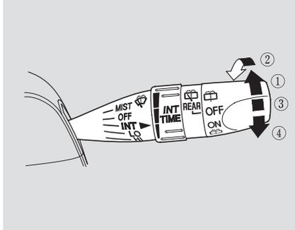
1. To turn on the rear window wiper, rotate the switch clockwise to ON. It operates intermittently.
