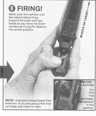
After the shot is fired, open the action, remove the fired round AND IMMEDIATELY RESET THE EXTERNAL FIRING PIN SELECTOR TO SAFETY POSITION 2. At all times, except for the instant before and after firing this selector must be set in safety position 2. NEVER CLOSE THE ACTION ON A LOADED ROUND UNTIL YOU HAVE CHECKED AND ASSURED YOURSELF THAT THIS SELECTOR IS SET IN ITS SAFETY (UNARMED) POSITION.
