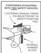
The Contender is equipped with two safety devices which function independently of each other (1. Safety position on the External Manual Firing Pin Selector. 2. Internal Hammer Block). When the Contender action is broken open properly, as explained on pages 5 and 6, the hammer block moves up into a position between the hammer and the frame. In this position the hammer cannot move forward
