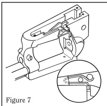
5. Insert the base pin. *The base pin must be fully inserted and locked in position by the base pin latch. If the base pin is not fully inserted and locked, the transfer bar may catch under the firing pin when the hammer is being cocked.*
