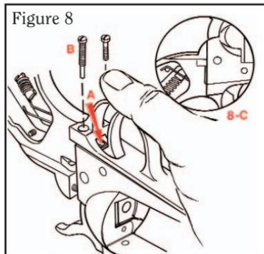
12. Hook the two ends of the trigger spring over the trigger spring retaining pin (KMVQ06300) as shown in Figure 8-C.
