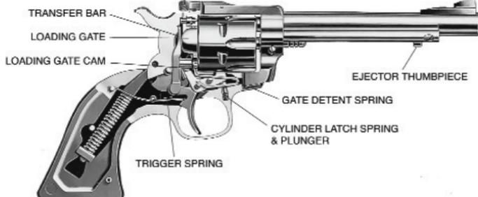
Mechanism shown at rest. Transfer bar is not in line between hammer and firing pin. This is the carrying position.
