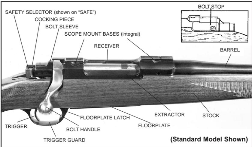
**Figure 1.** Right-handed version shown. In this illustration the cocking piece is shown cocked (protruding from the rear of the bolt sleeve). The bolt stop (on the left side of the receiver) permits the bolt to be withdrawn simply by pulling it out to the left. The safety selector should be in the “Load-Unload” position when the bolt is being removed or installed.
