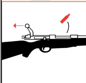
When firing the M-77® Mark II be sure that bystanders are well clear of the shooter and standing a safe distance to the rear. Empty cartridge cases are hot and are normally ejected from the rifle to the right. They could cause injury to any person who is standing too closely alongside the shooter. Shooters who fire right-hand rifles from their left shoulder should be particularly cautious concerning ejected cartridge cases and the back of the bolt as it is drawn rearward.
