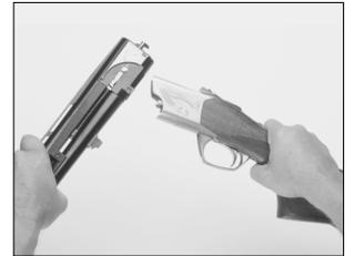
Engage the receiver into the MonoLock Hinge's circular arc.
