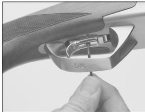
Remove the center trigger screw with an Allen wrench.
