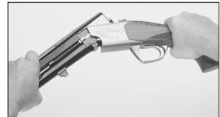
Push and rotate the receiver until it fully engages and locks into the barrel set.
