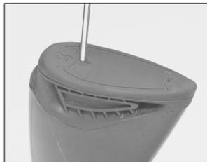
Locate the entry holes in the end of the recoil pad.
