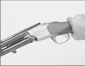
If the receiver is not engaging the barrel set, do not force it. Remove the receiver and start over.
