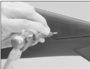
To remove the comb, tap out the pin with a punch or drift pin, then slide the comb *forward* off the ribs.
