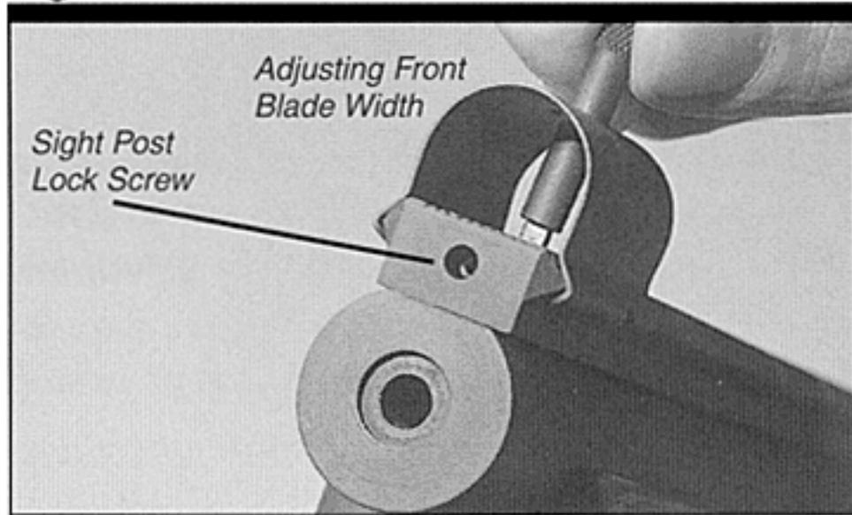
**BLADE WIDTH**— To increase or decrease the width of the blade, loosen the front set screw found on the front of the top sight rib (above the muzzle) with the 1/16" Allen wrench (supplied). Insert the slotted front sight adjusting wrench (supplied) into the access hole at the top of the sight hood and rotate the blade up to 90 degrees, to the desired width (See Figure 10). Retighten the set screw with the allen wrench.
