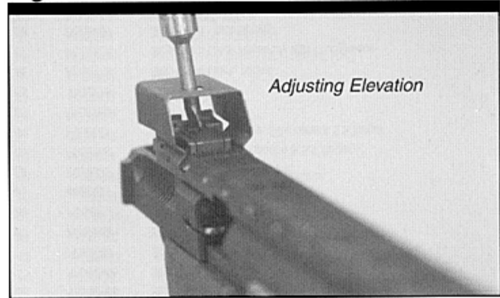
To move the point of impact to the left, turn the screw in a counterclockwise direction.
