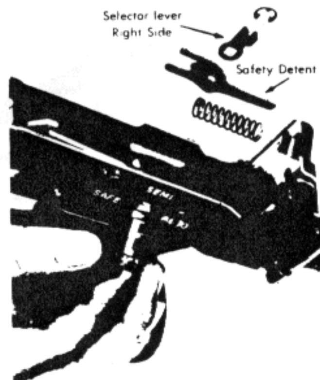
Disengage/Remove Selector Lever
