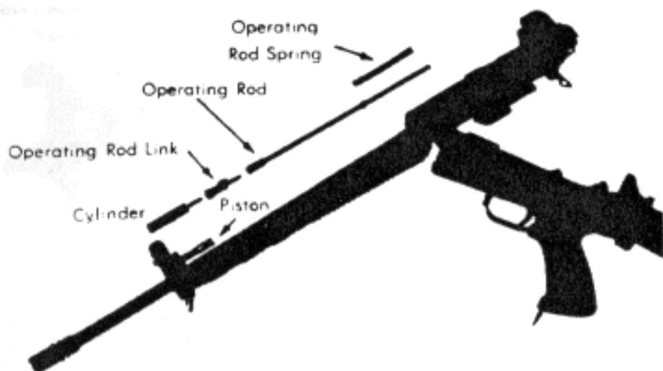
Remove/Install Operating Rod Assembly
