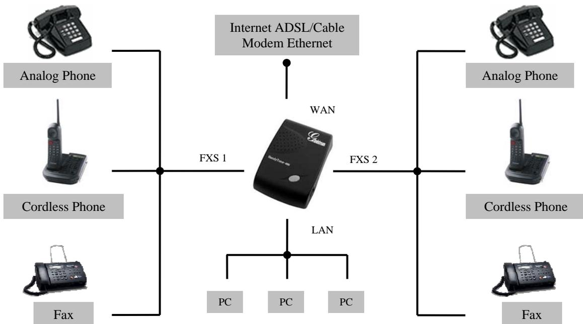
HandyTone-496 has two FXS ports. The PHONE1 port next to the LAN is FXS port 1 and the PHONE2 on the side of the HandyTone-496 is FXS port 2. Each FXS port can have a separate SIP account. This is a key feature of HandyTone-496. Both ports can make calls concurrently.
