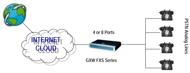
FXS Gateway acts as a 'virtual office', connecting analog lines directly to the gateway
