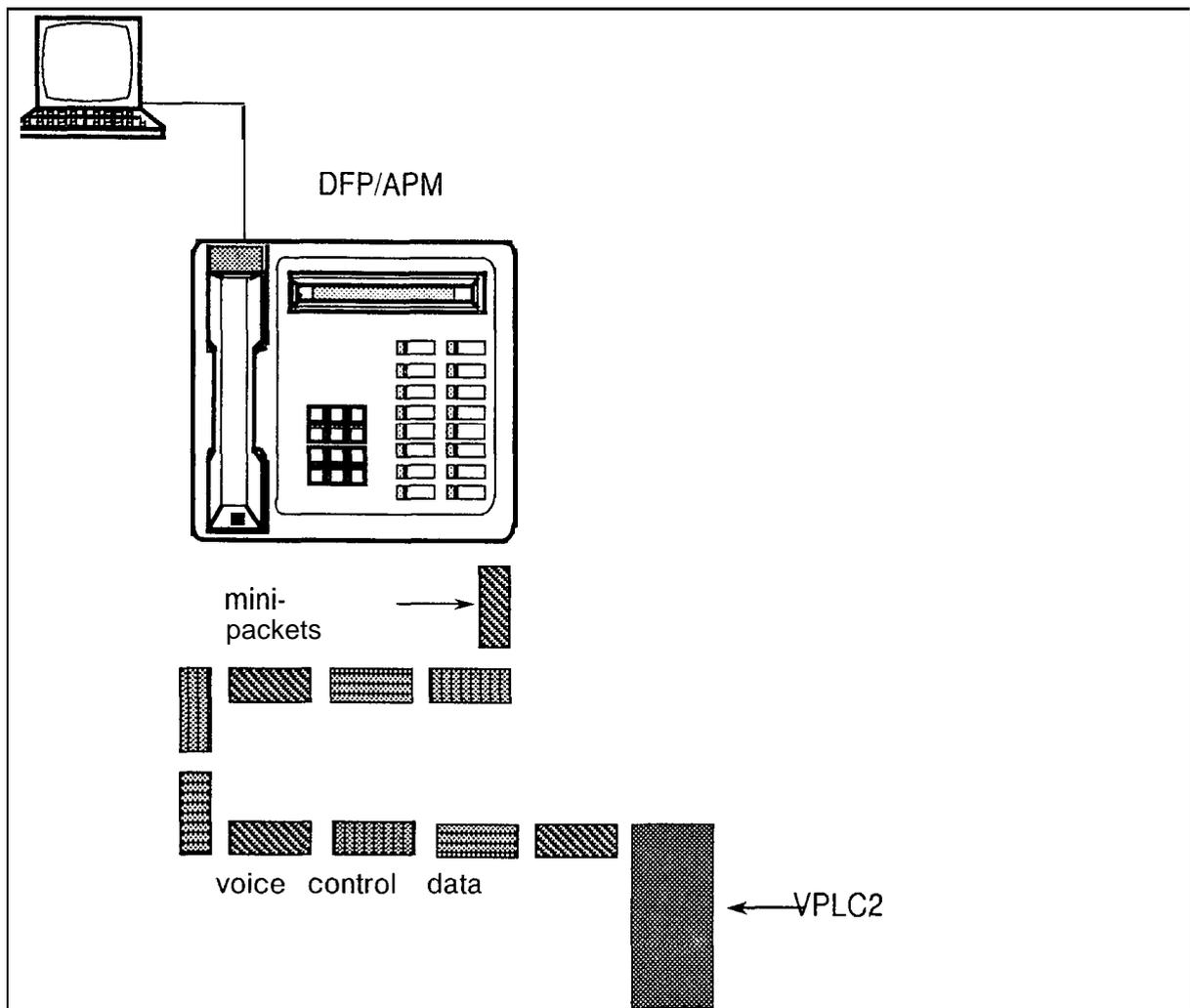
Figure 33.2 Transmission from the Digital Featurephone to the System
