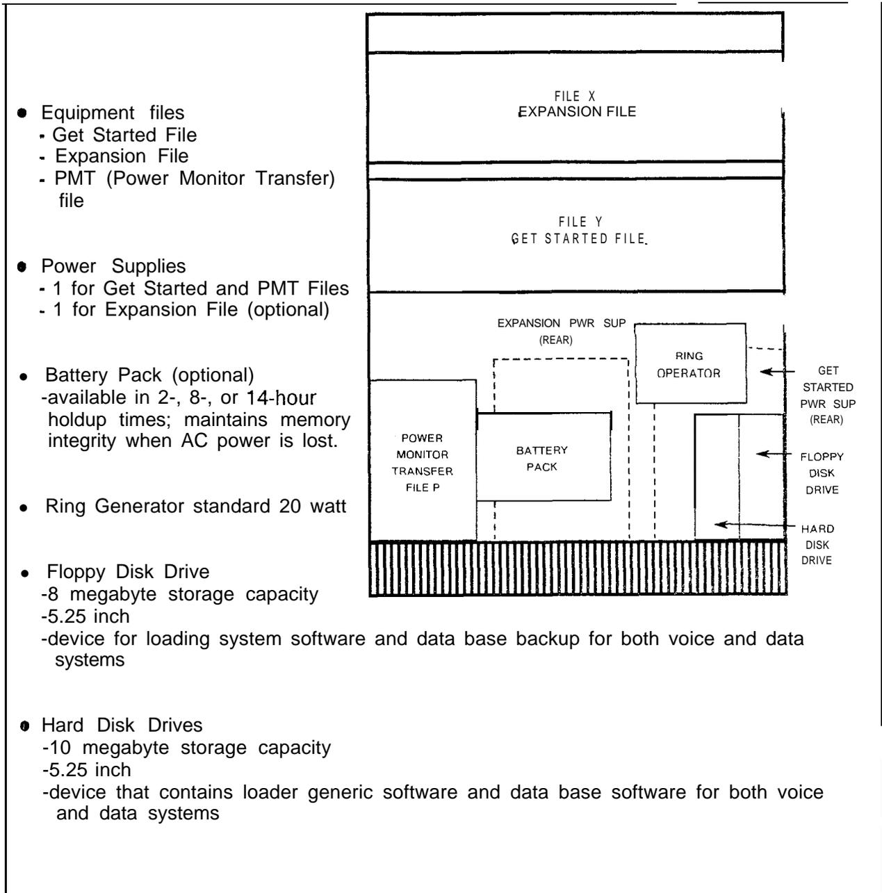
Figure 2.2 Equipment Cabinet Configuration
