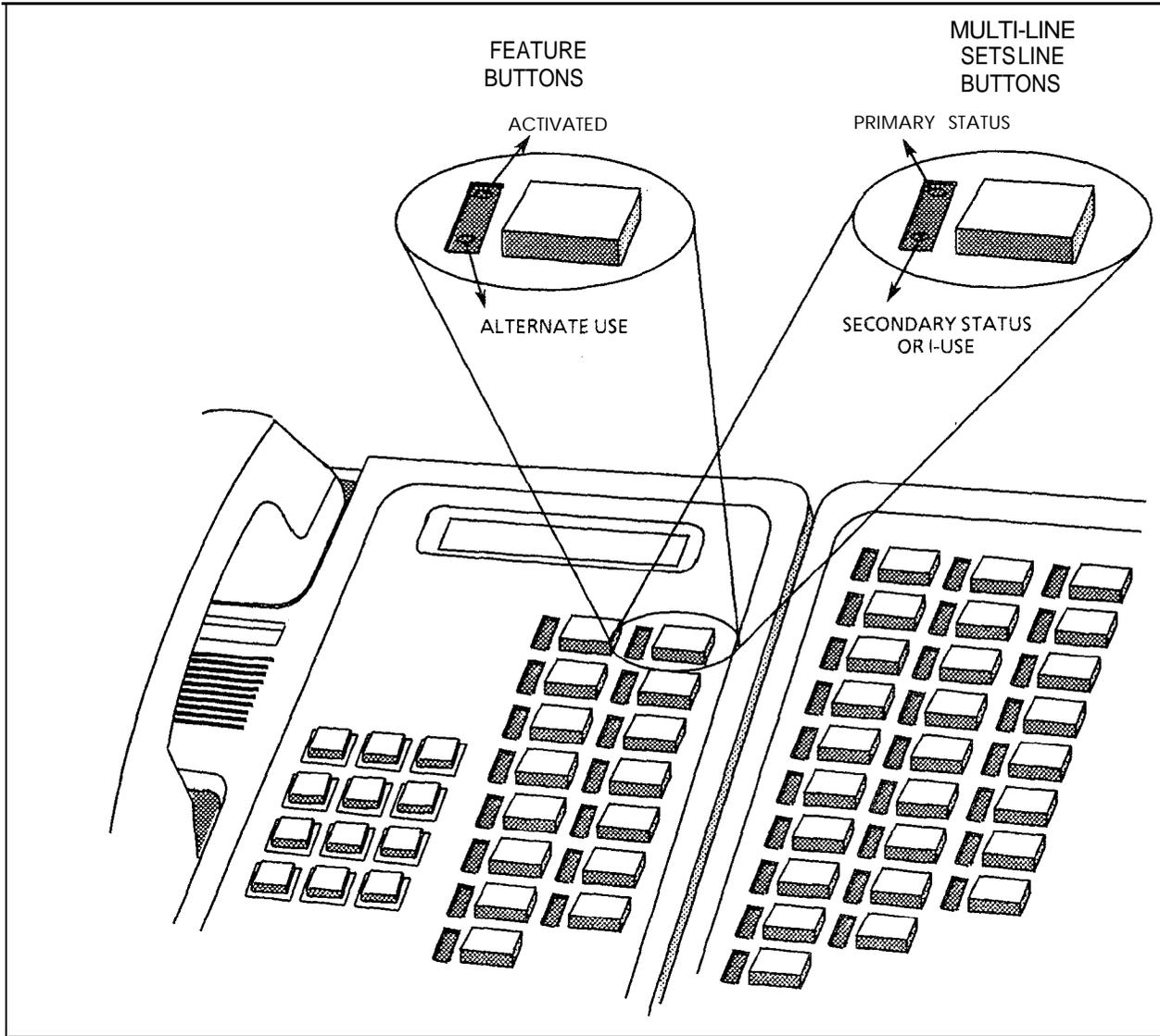
Figure 3.3 Integrated Featurephone Status and i-Use LEDs
