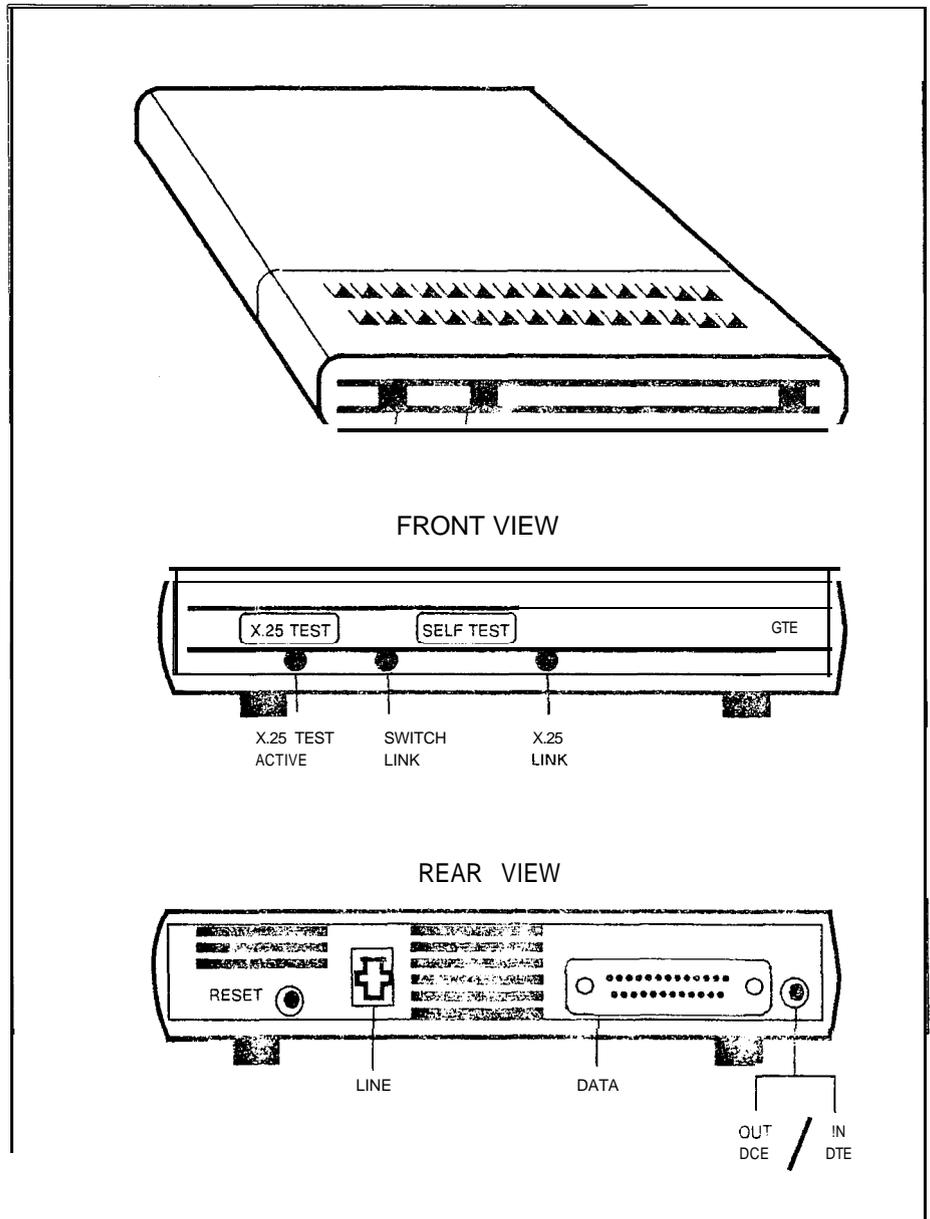
Figure 32.1 SPM (Synchronous Packet Manager)
