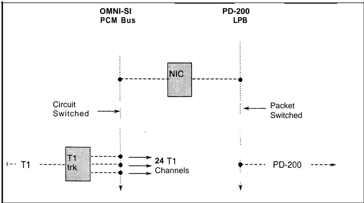
Figure 33.4 NIC Card within the OMNI SI System's Architecture
