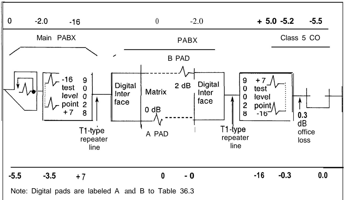
Figure 36.11 Intertandem Tie Trunk to CO Trunk Call (FLP)
