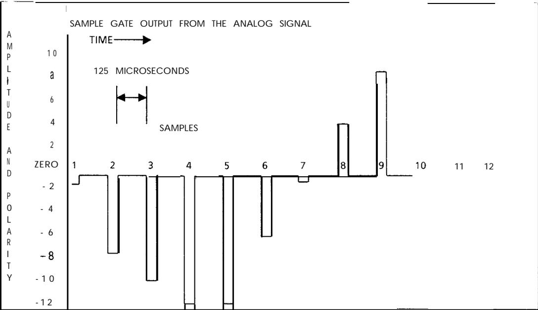
**Figure 4.7 Sampling an Analog Signal**
