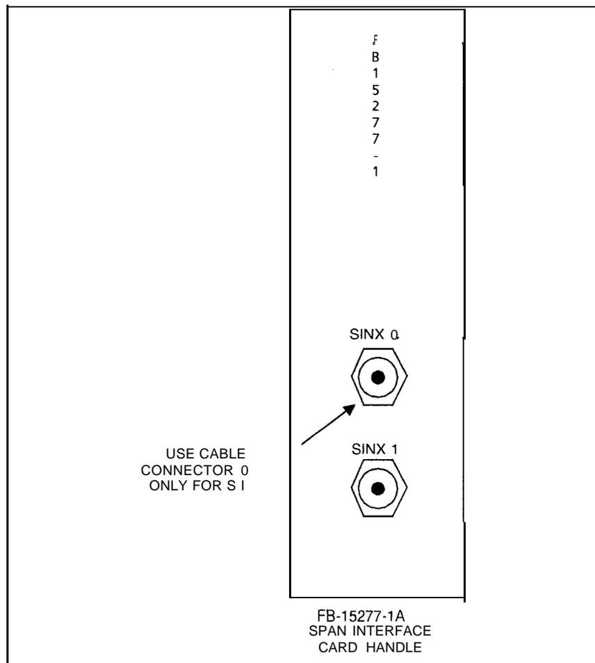
**Figure 29.3 FB-15277-1A Span Interface Card Handle**
