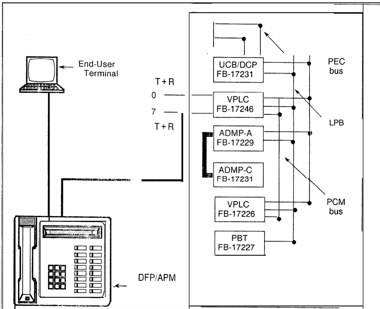
Figure 33.1 DFP/APM Voice and Data Bus Connection
