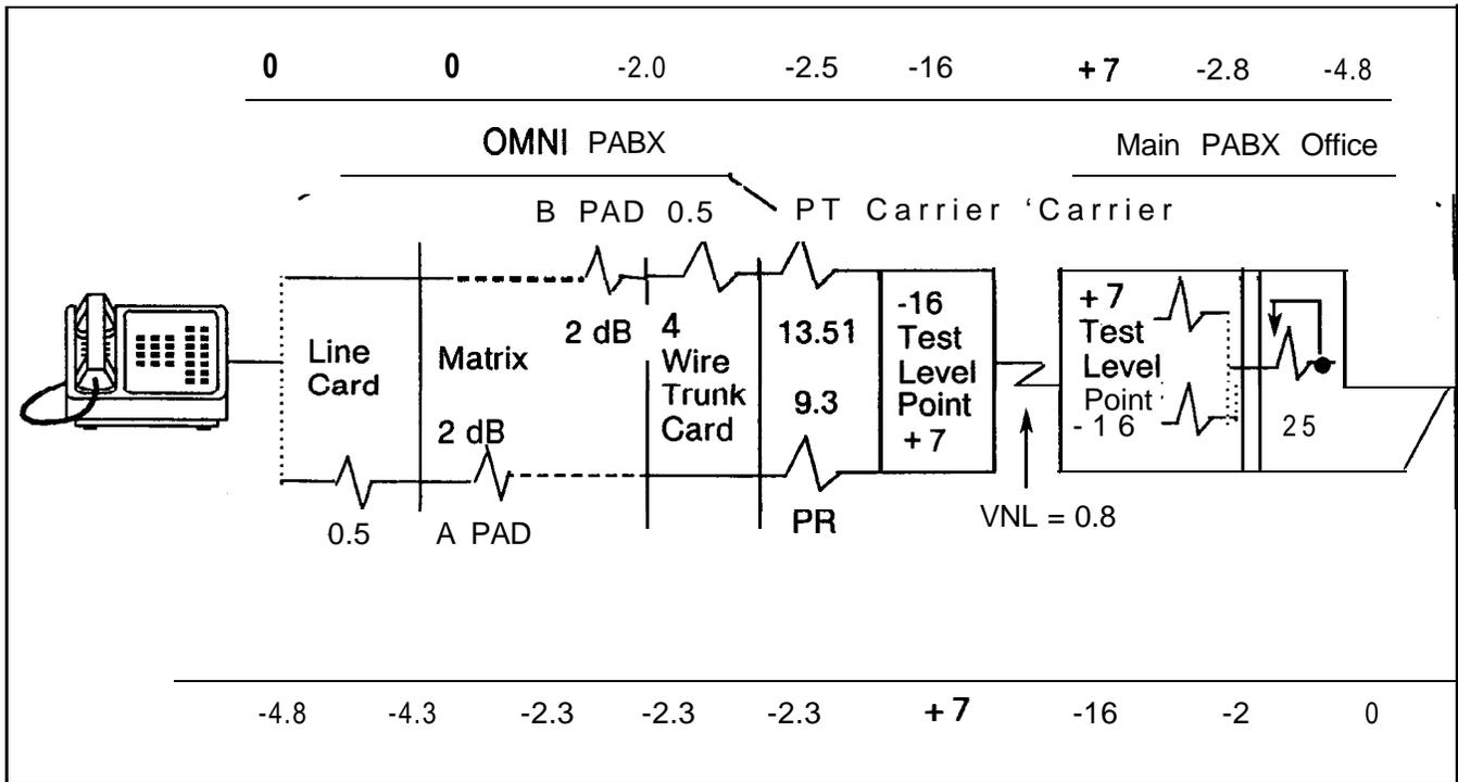
Figure 36.3 Line to Intertandem Tie Trunk Call (VNLP)
