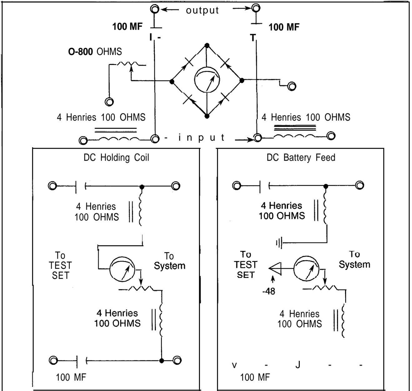
Figure 36.12 Hold Coil and Battery Feed Arrangements
