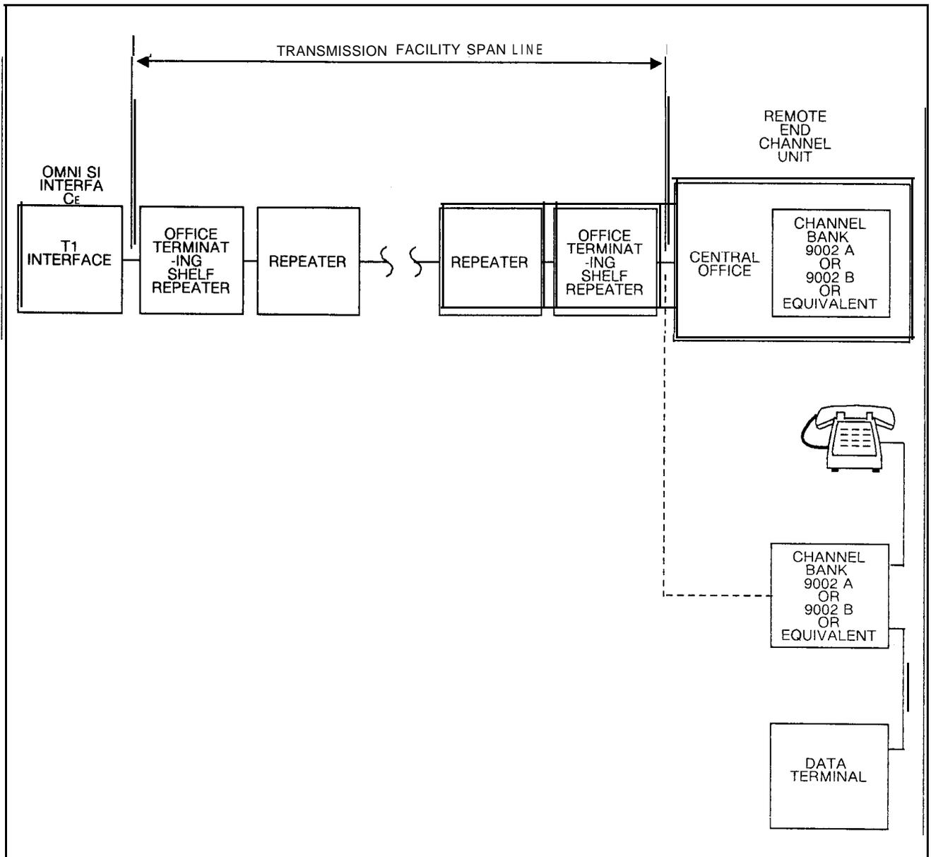
Figure 29.1 T1-Type Digital Trunk Link
