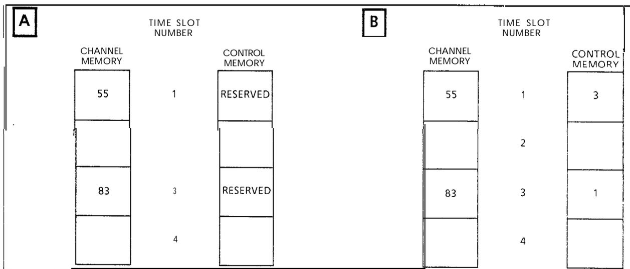
**Figure 4.5 Time-Switch Memory Setup**
