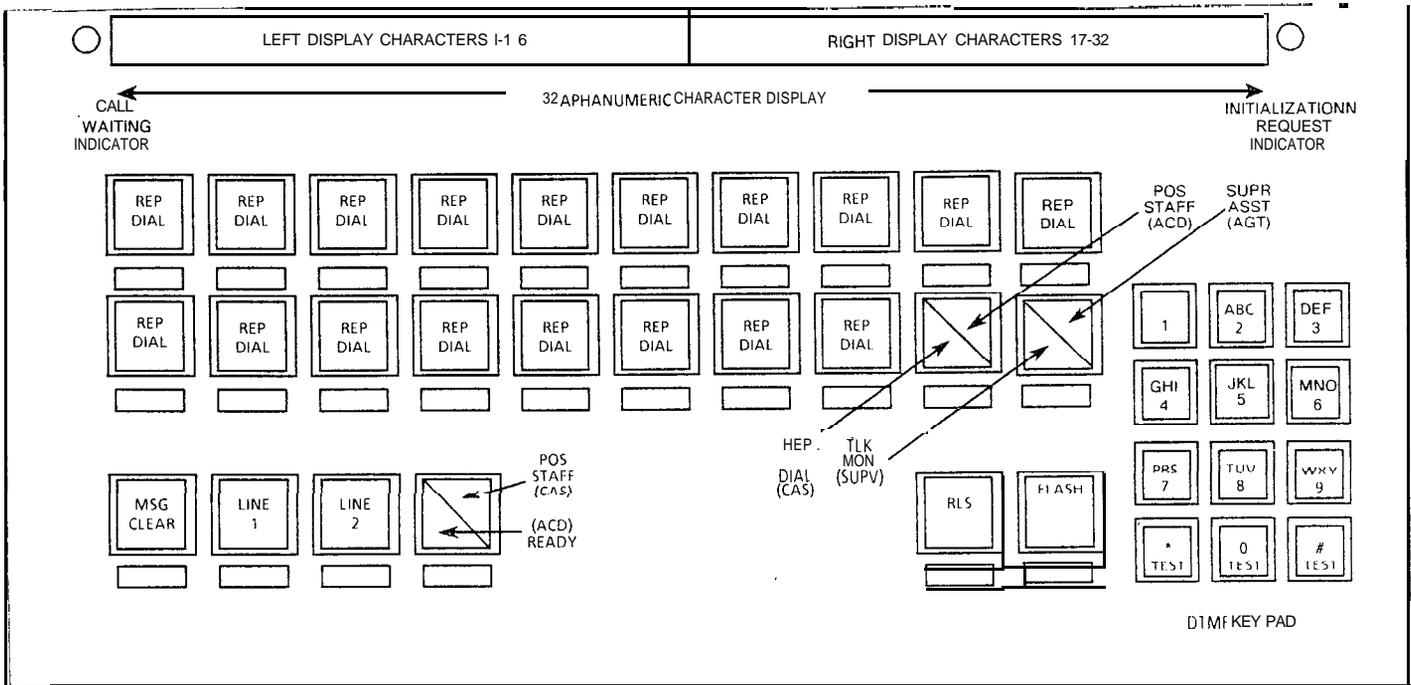
Figure 17.6 Agent Instrument Controls and Indicators
