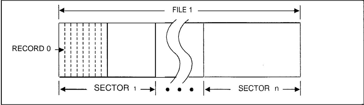
Figure 4.16 Disk File Breakdown
