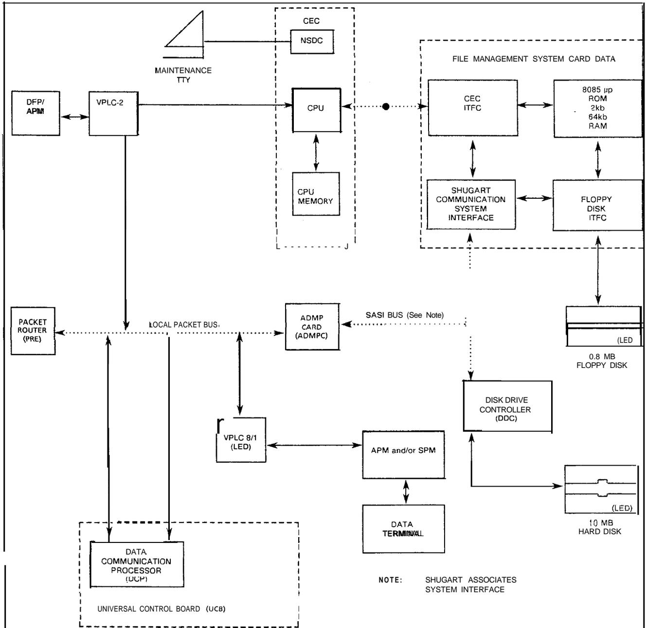
**Figure 8.2 Simplified Disk System Interface**
