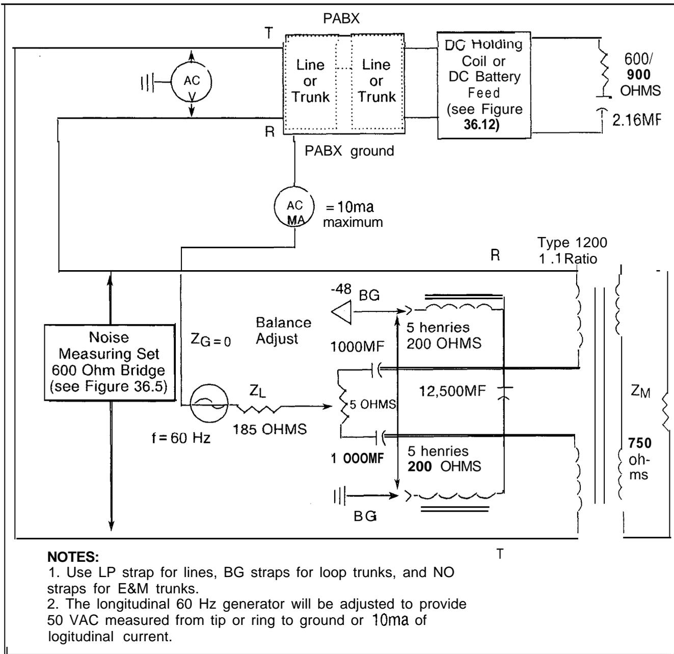
Figure 36.17 Longitudinal Susceptibility Measurement
