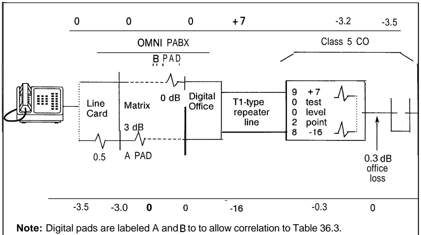
Figure 36.8 Line to CO Trunk Call (FLP) with T1-Type Repeater Line
