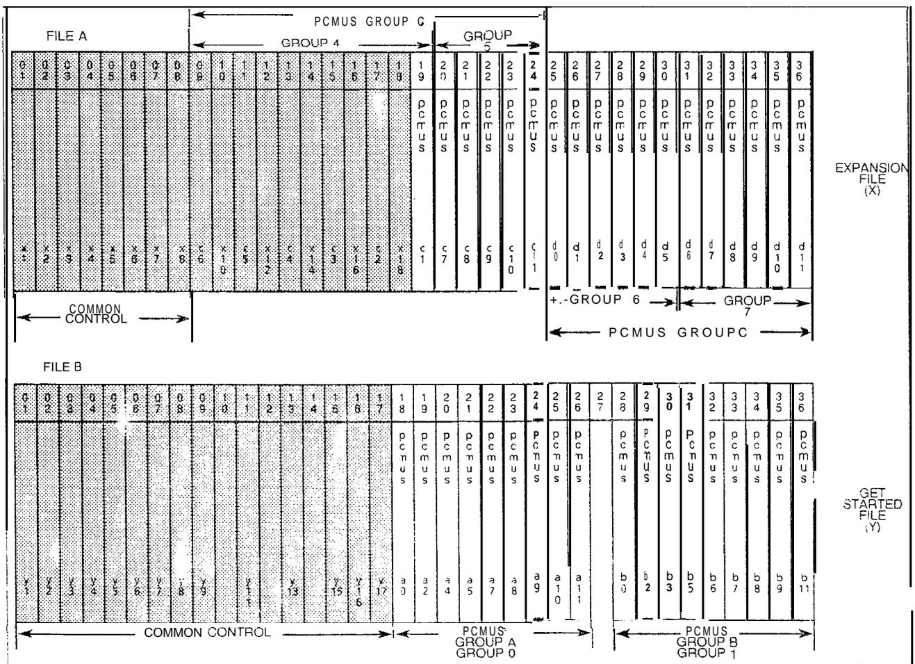
Figure 7.1 Universal PC8 Card Slots Used by PD-200 Cards
