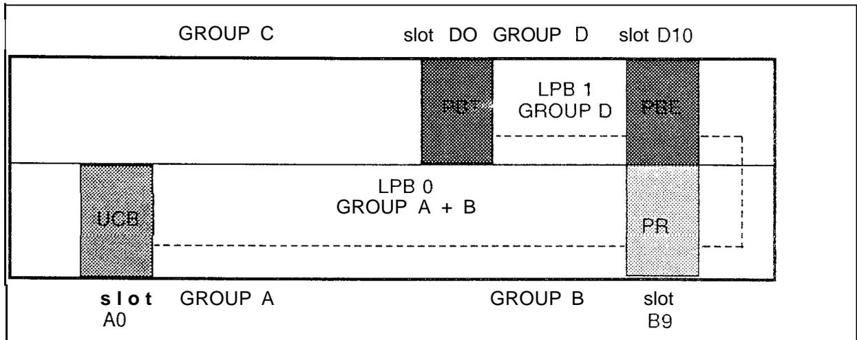
Figure 12.5 Example of Two Local Packet Buses (LPB 0, LPB 1) in Groups A & B and D
