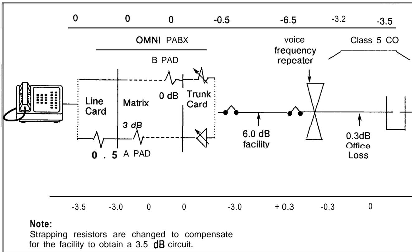
**Figure 36.6 Line to CO Trunk Call (FLP) with Voice Frequency Repeater**
