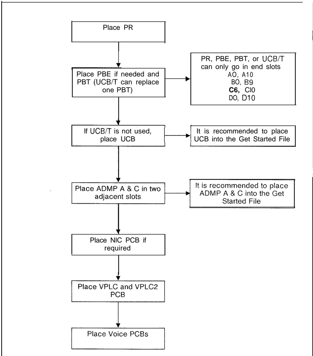
Figure 12.7 Flowchart for Card Placement
