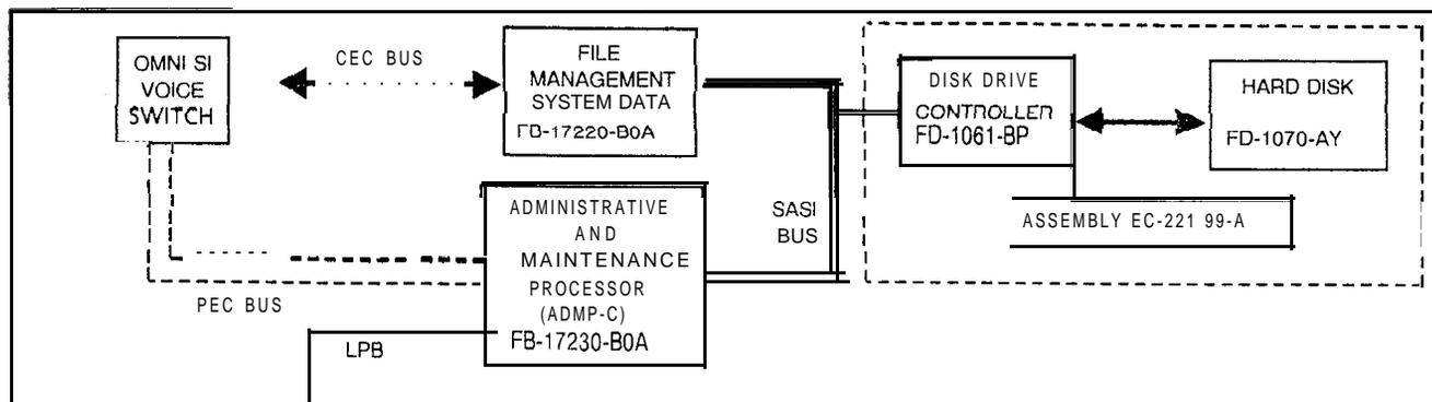
Figure 8.3~ FMSD and Hard Disk Assembly Interface
