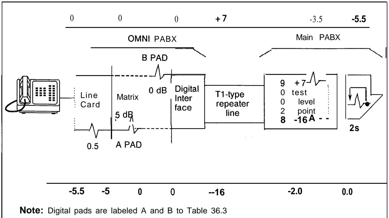
Figure 36.10 Line to Intertandem Tie Trunk Call (FLP) with TI-Type Repeater Line
