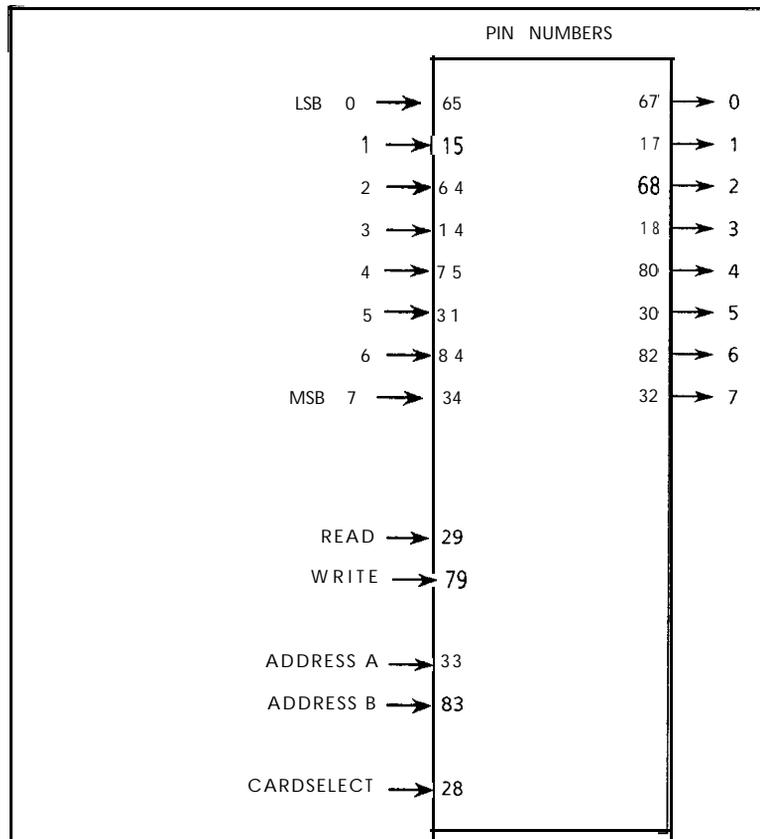
Figure 4.2 Control and Sensing Connections of PCI Universal Slot
