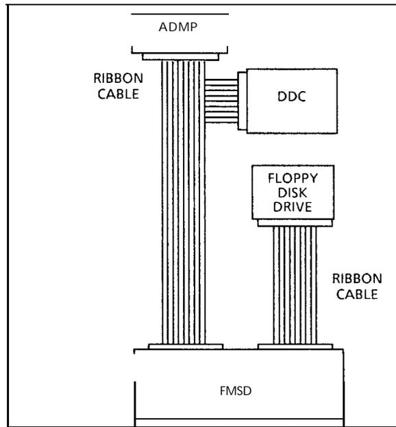
**Figure 8.4 Disk System Cabling**
