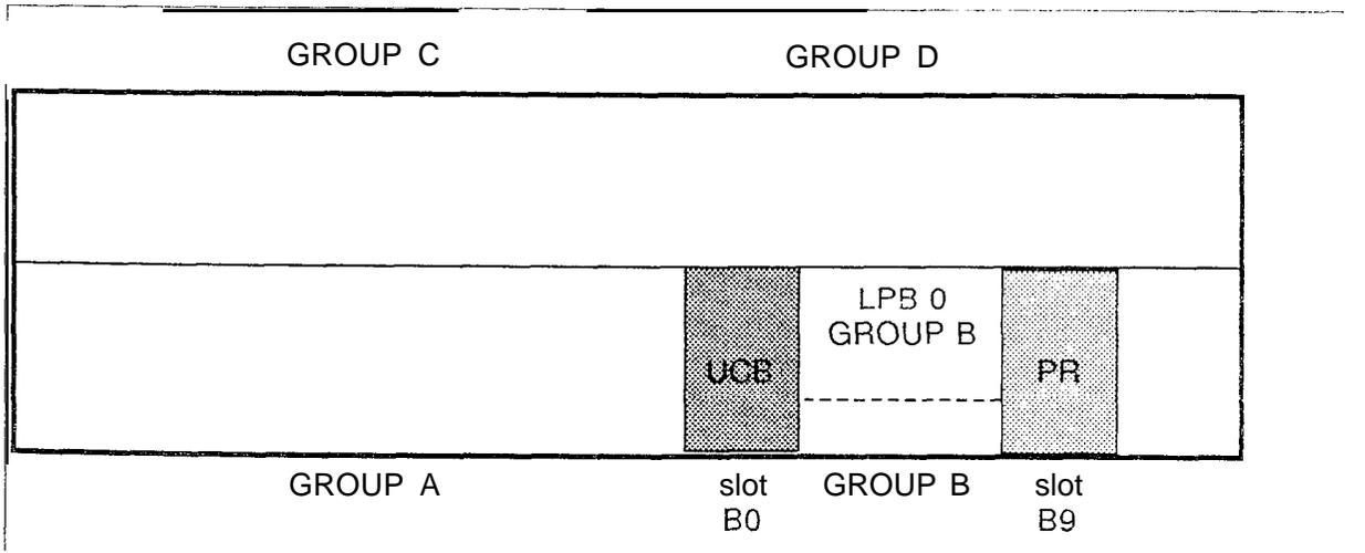
Figure 12.3 Example of Single Local Packet Buses in Group B
