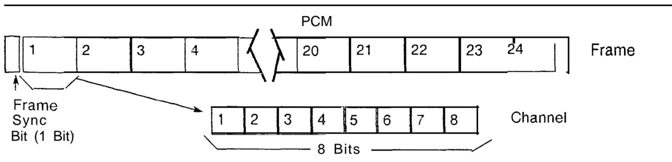
**Figure 5.2 PCM (Pulse Code Modulation) Bus**
