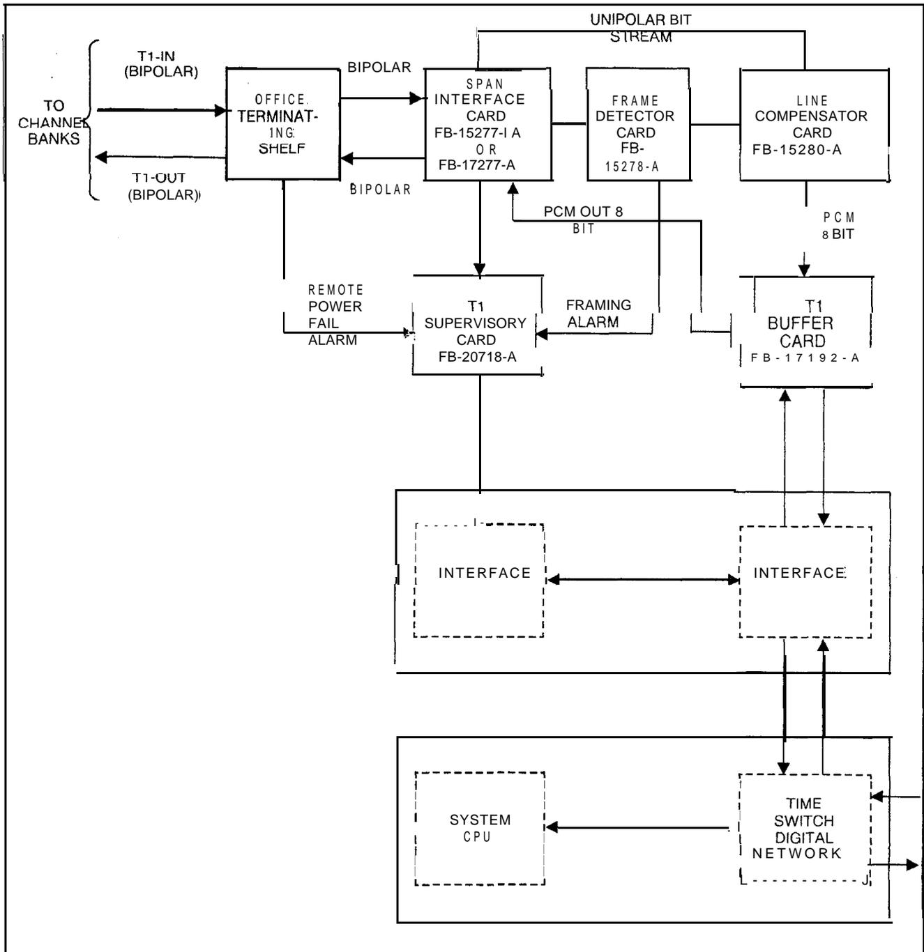
Figure 29.2 T1 Digital Trunk Interface in the System
