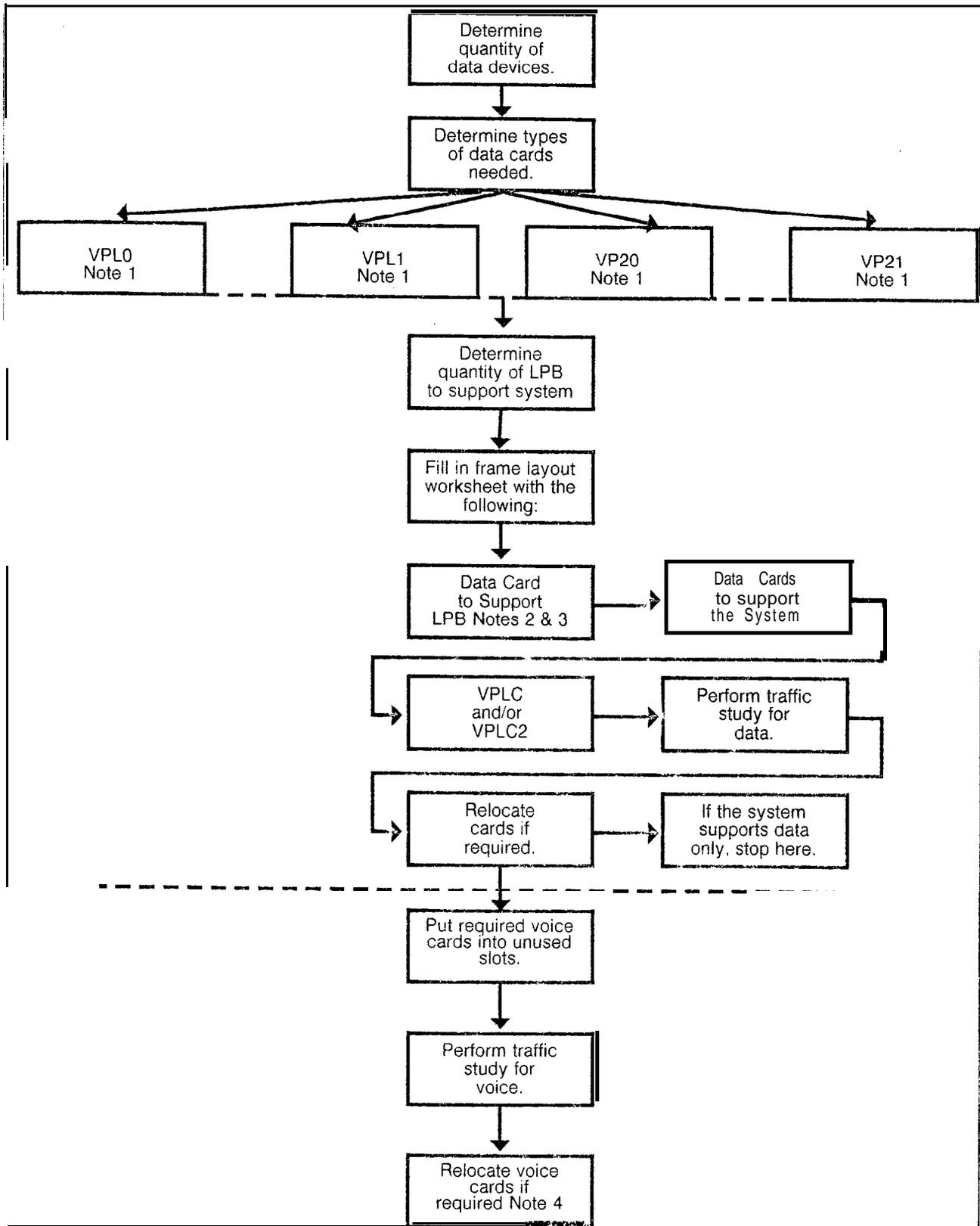
Figure 13.1 Flowchart for Configuring the System
