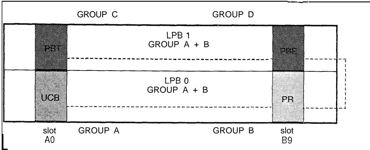
Figure 12.2 Example of Two Local Packet Buses (LPB 0, LPB 1) in Groups A & B, C & D
