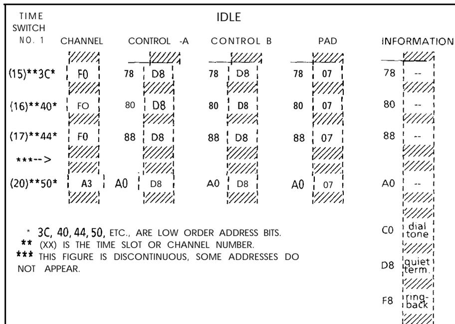
**Figure 34.2 Time-Switch memories During Idle**
