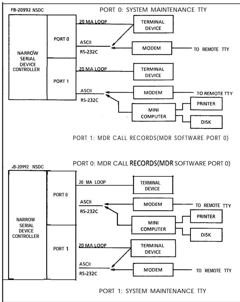
Figure 6.1 Possible NSDC Port Assignments with MDR Port 0 (Call Records) Equipped in Data Base
