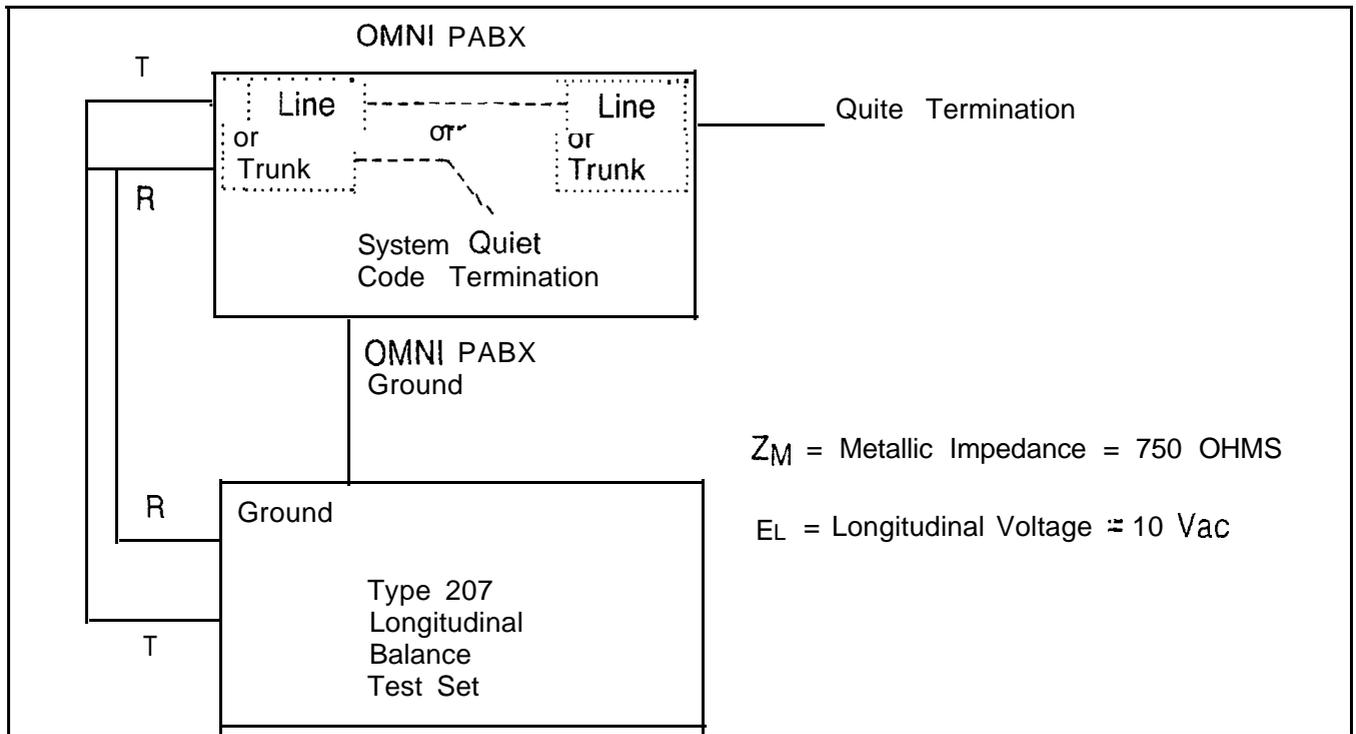
**Figure 36.16 Longitudinal Attenuation Measurement**
