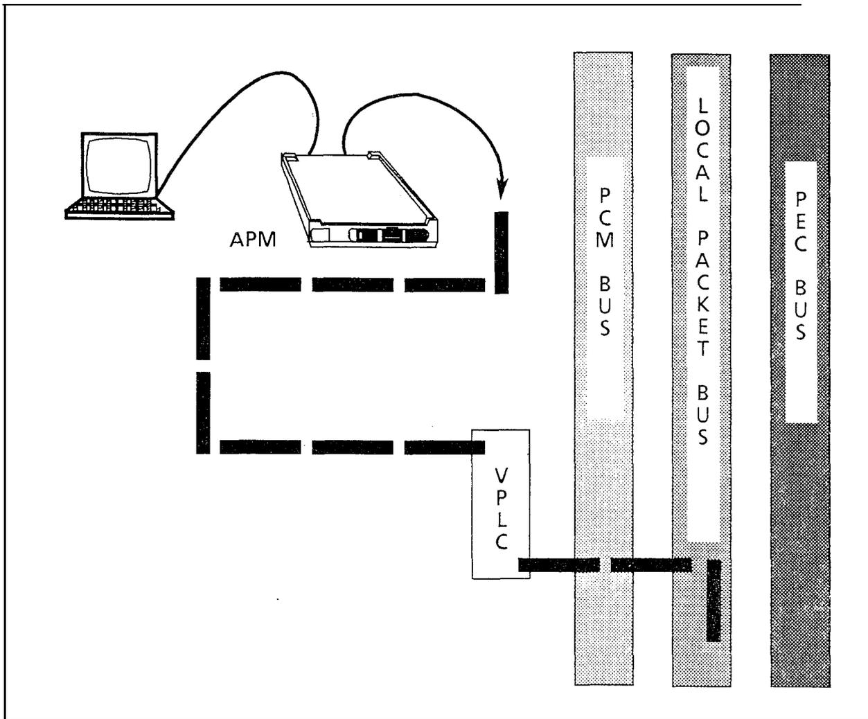
Figure 8.5 Transportation of Mini-Packets over LPB
