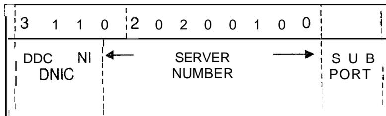
Figure 9.7 Example of Load Sharing Numbering Plan
