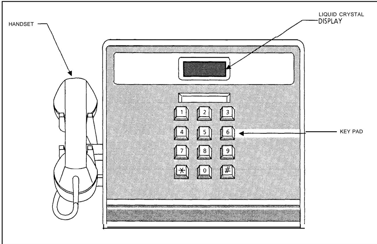
Figure 17.1 Display Telephone
