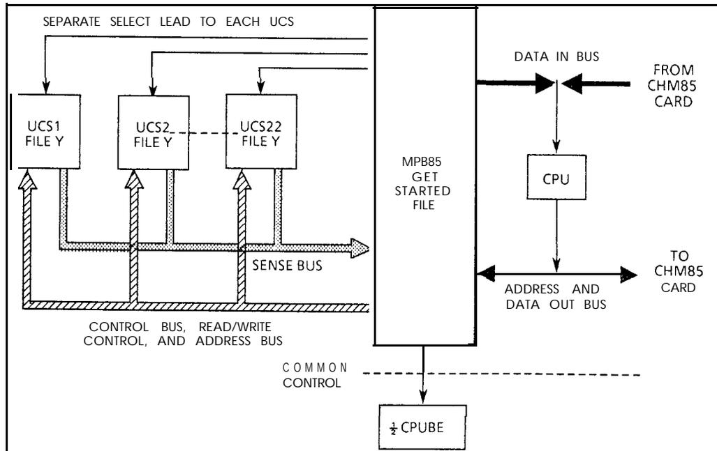
Figure 4.3 Common Control Related Circuits
