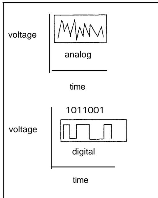
**Figure 10.1 Analog and Digital Signals**
