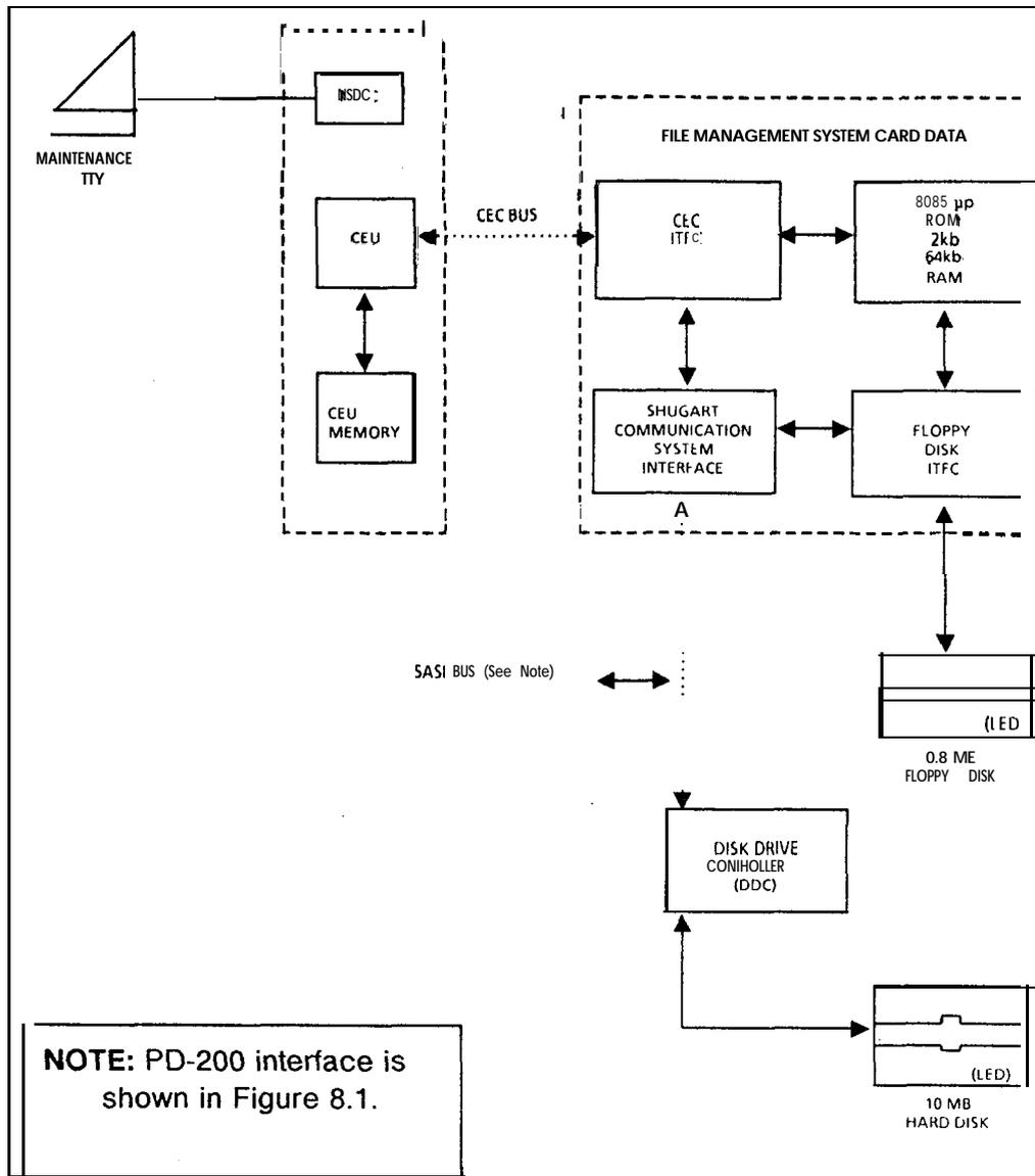
Figure 4.13 Simplified Disk System Interface
