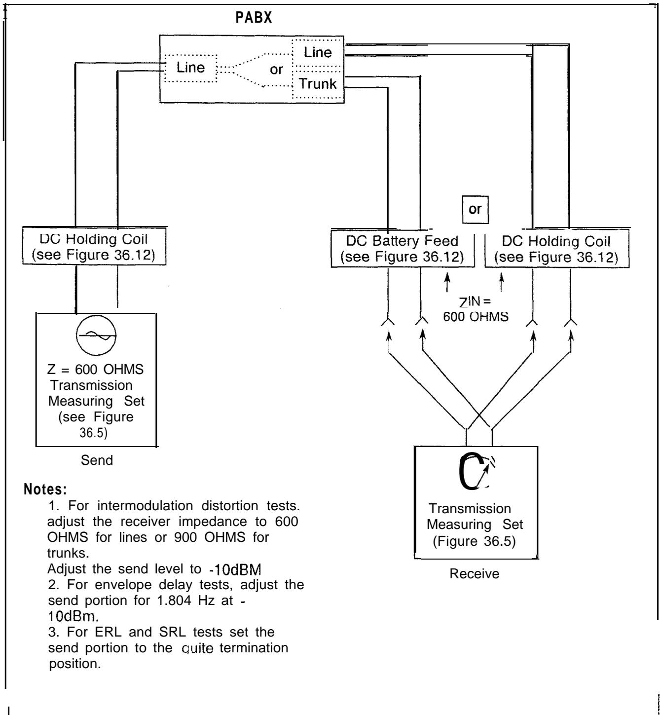
**Figure 36.18 Intermodulation, Envelope Delay Distortion, Noise, and Return Loss Test Method**
