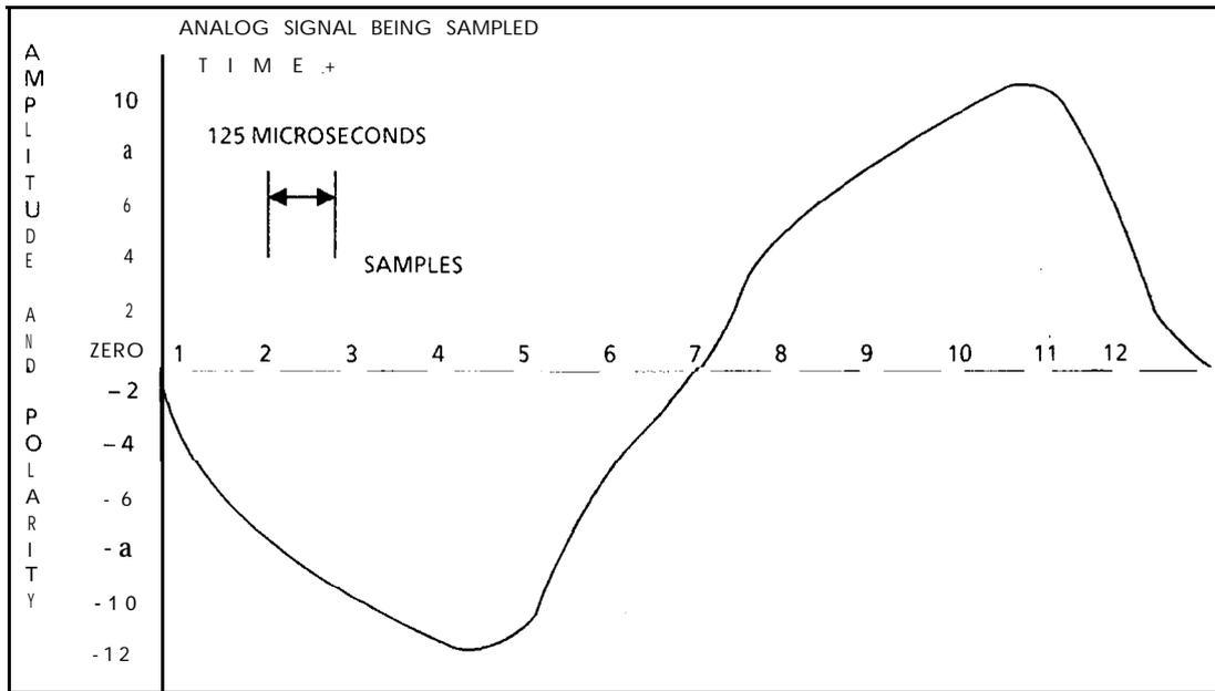
Figure 4.8 Sampling an Analog Signal
