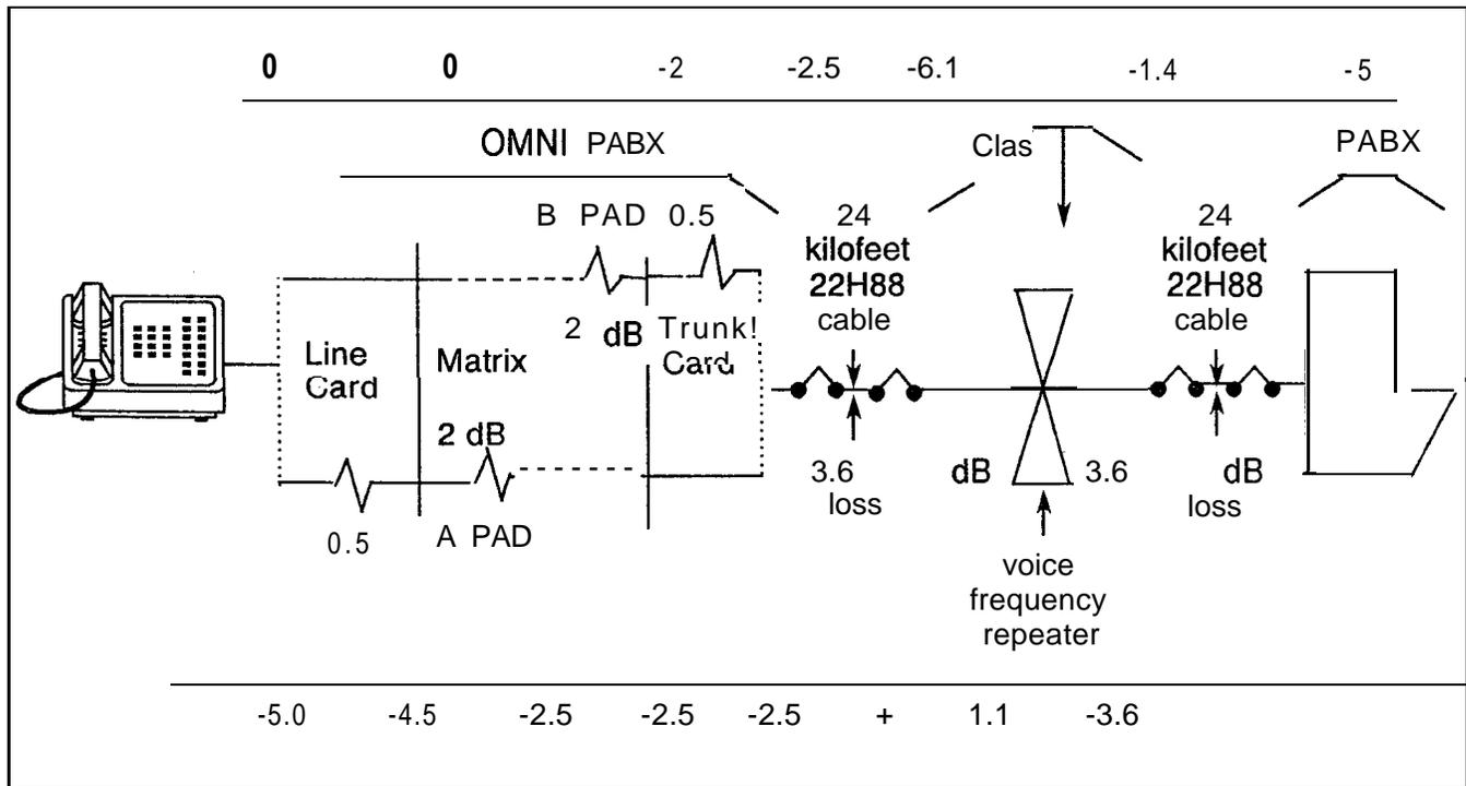
Figure 36.4 Line to Nontandem Tie Trunk Call (VNLP)
