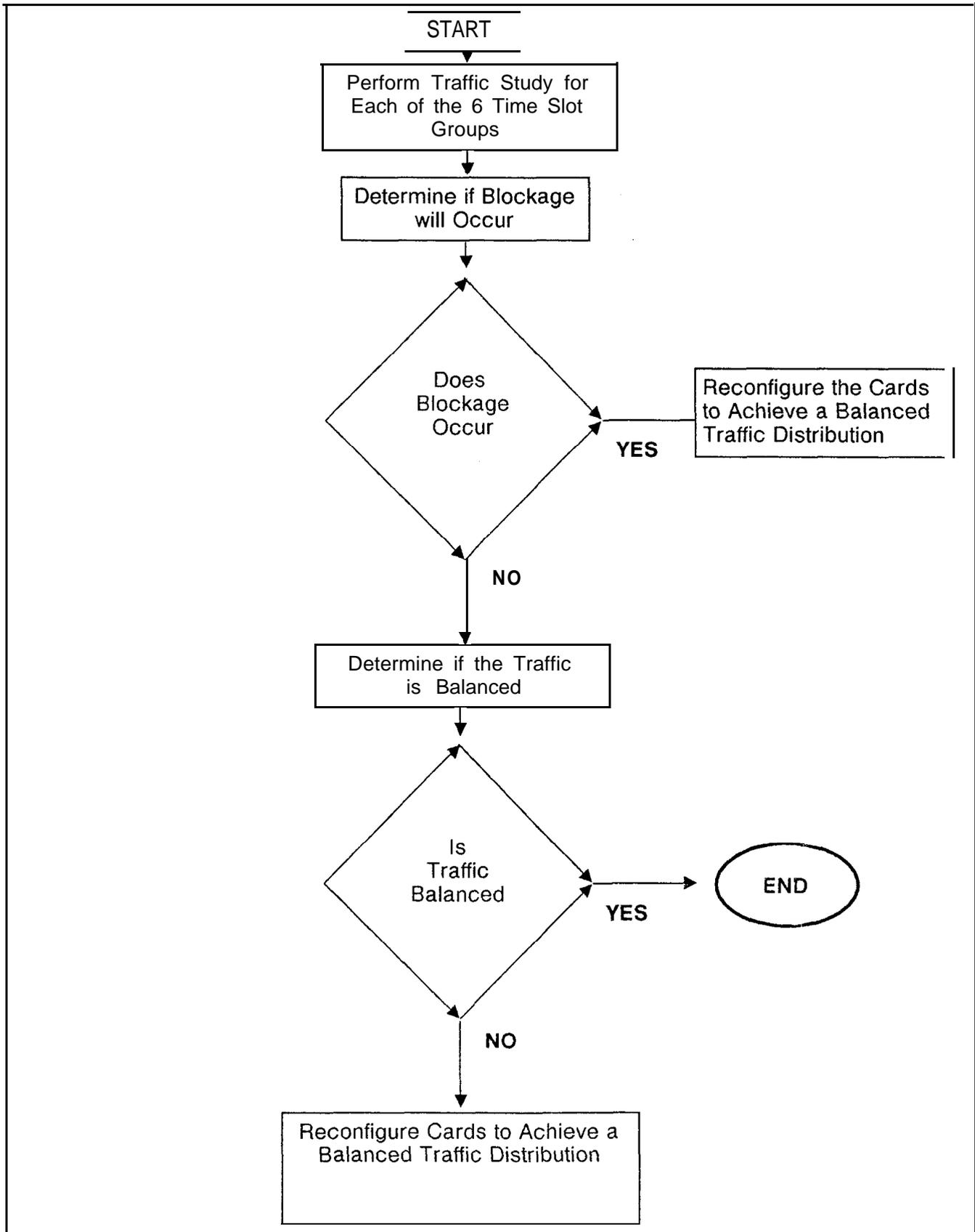
Figure 11.1 Flowchart for Balancing System Traffic
