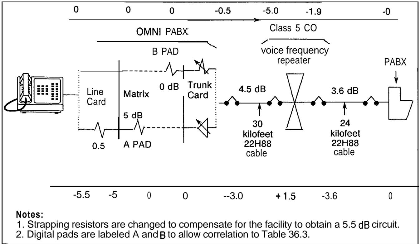
Figure 36.7 Line to Nontandem Tie Trunk Call (FLP)
