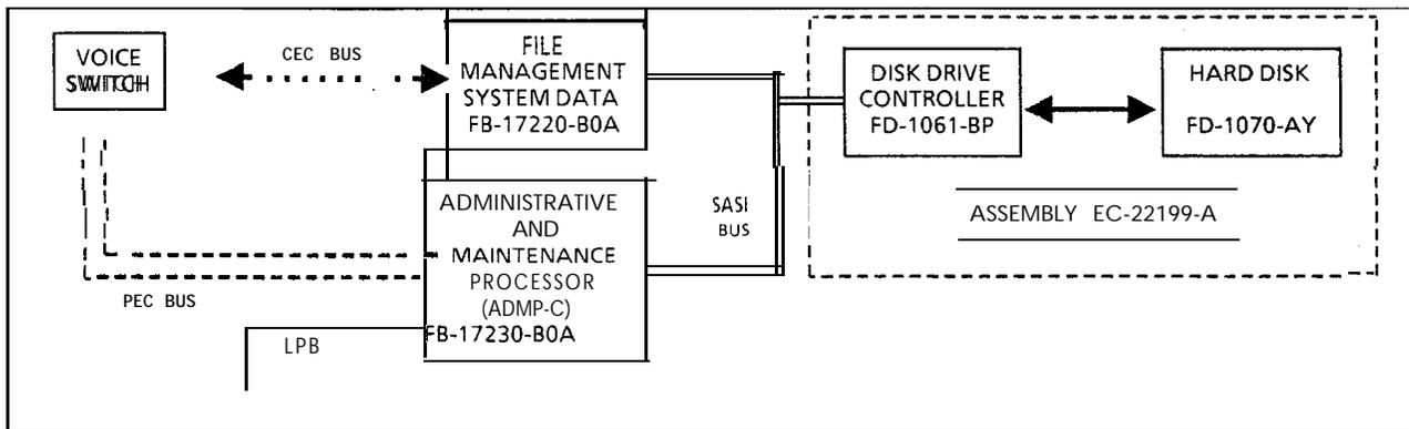
**Figure 6.2 Data System Access to Mass Storage**
