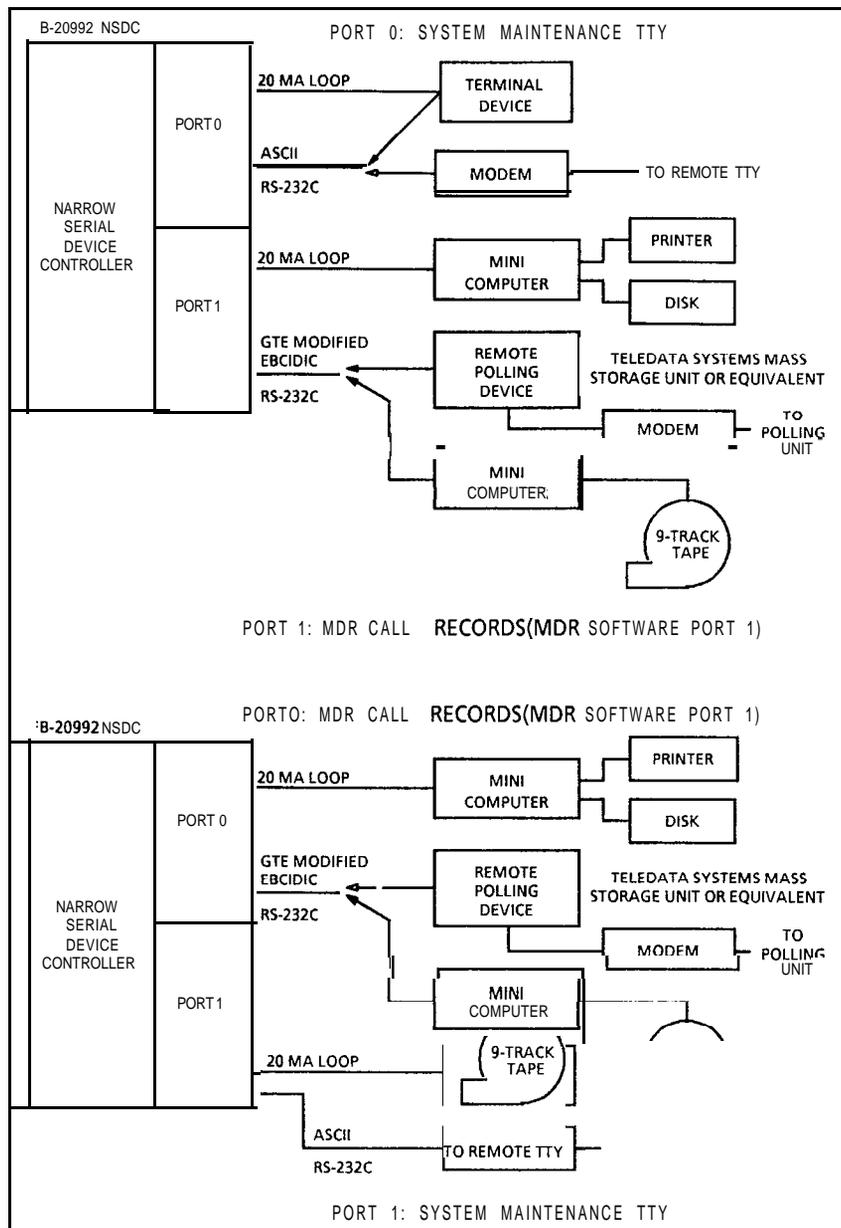
Figure 6.2 Possible NSDC Port Assignments with MDR Port 1 (Call Records) Equipped in Data Base
