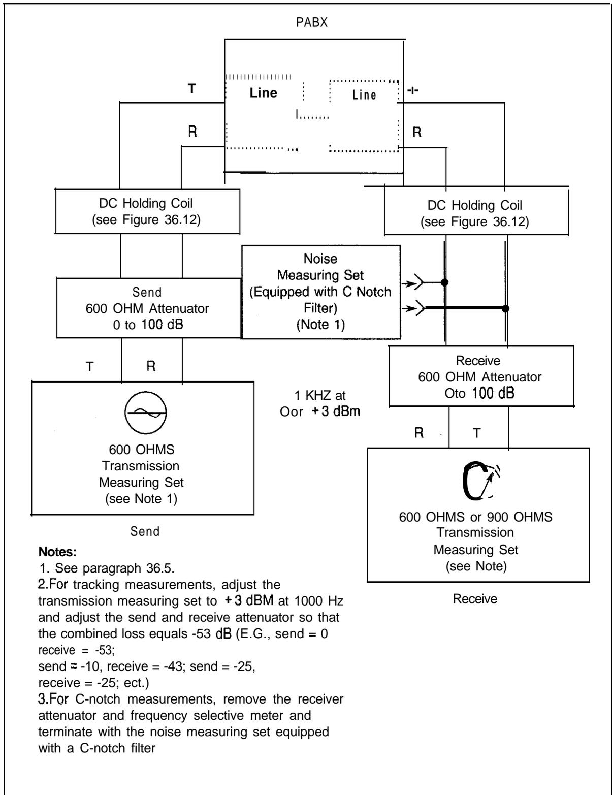
**Figure 36.14 Level Tracking and C-Notch Distortion Measurement**
