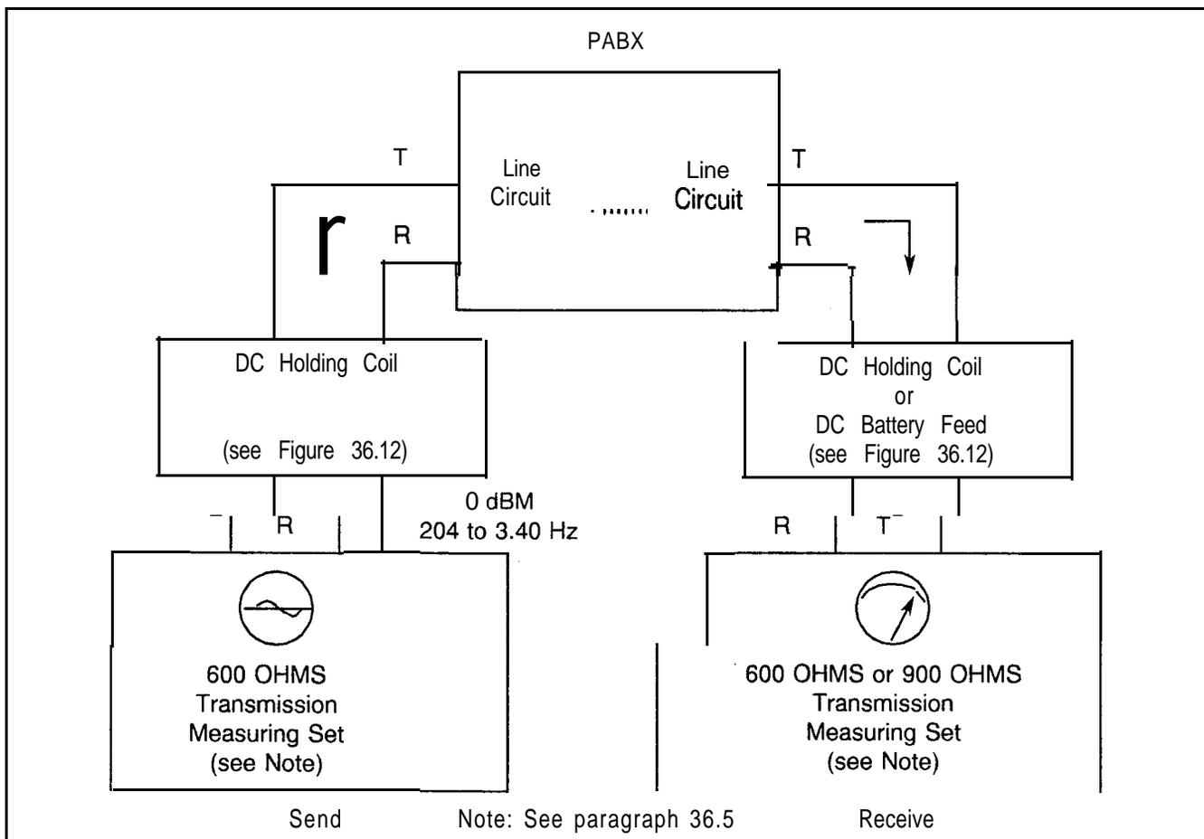
**Figure 36.13 Insertion Loss and Frequency Response Measurement**
