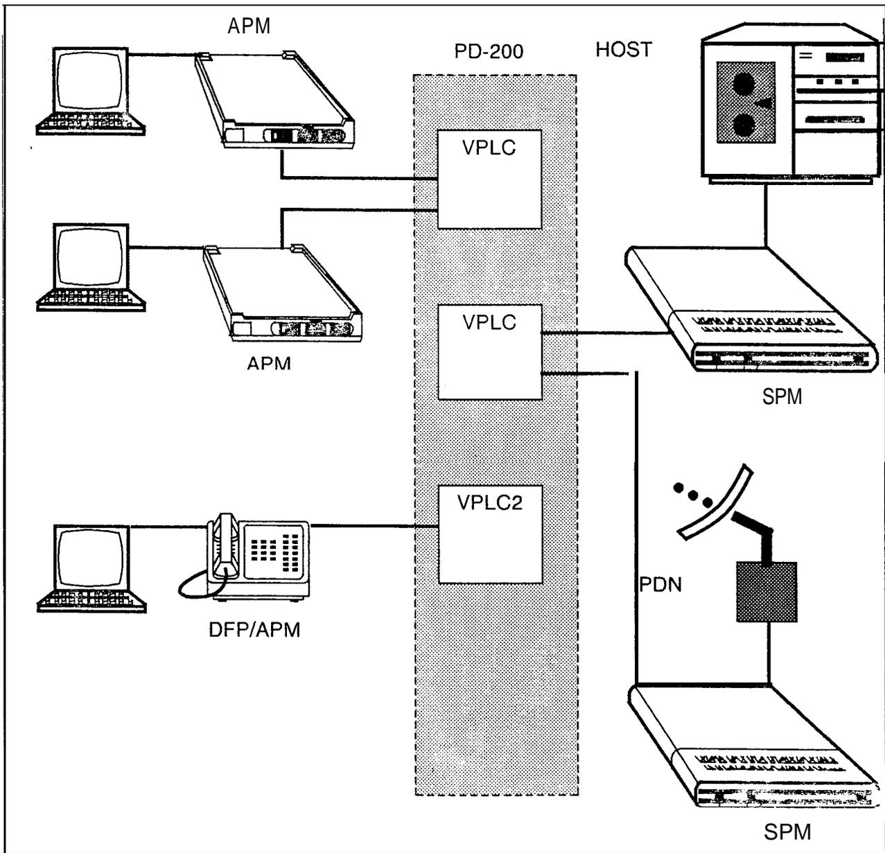
Figure 6.5 Remote Processor/VPLC (Voice Packet Line Card) Connection
