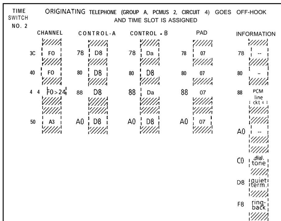
Figure 34.3 Off-Hook Time Slot Assignment
