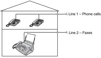
Only a fax machine is connected.
