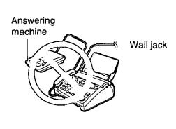
Do not connect an answering machine when using the TEL/FAX mode.
