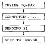
If the number you dialed is out of the FaxSav network service area, the unit will show the following messages and send the fax directly over the telephone line.
