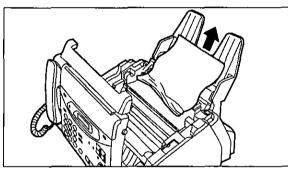
If the film is slack, turn the film cartridge over and tighten it by winding the gears.
