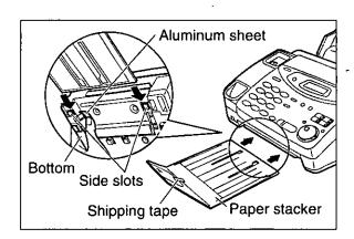
Confirm that the paper stacker is locked into the center slots and slide back.
