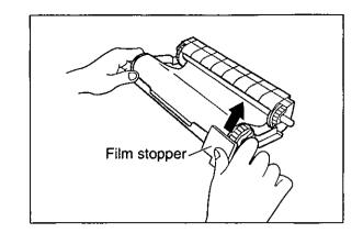
If the film is slack, tighten it by winding the gears.
