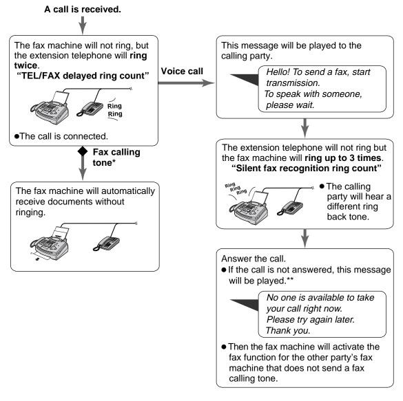
\* A fax calling tone is automatically generated by the sending fax machine. Some fax machines do not have this capability.
