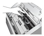
*Tip!* If the cartridge carriage moves back to the side before you put the cartridge in, shut and re-open the print cartridge doors.
